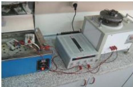
**Figure 1: Laboratory system used to synthesize the lead dioxide nanoparticles, including power supply, pulse maker apparatus, and electrochemical cell**
