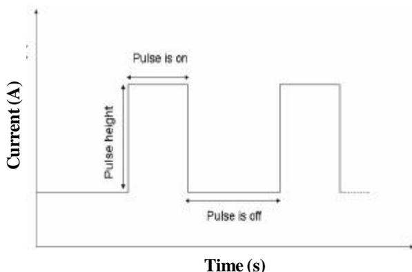
**Figure 2: Used pulse diagram, including pulse time, relaxation time, and pulse height**
