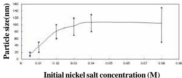
Figure 7: Effect of the initial nickel salt concentration on the average and range of nickel particles size
