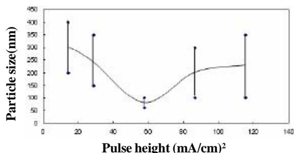
**Figure 4: Effect of the pulse height (current density) on the average and range of nickel nanoparticles size**
