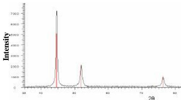
Figure 10: XRD patterns for the optimized nickel nano powder sample
