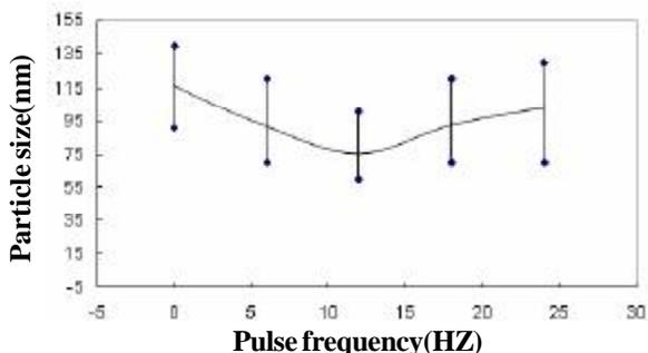
**Figure 3: Effect of the pulse frequency on the average and range of nickel nanoparticles size**
