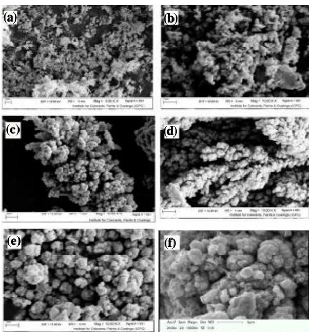
Figure 6: SEM images of nickel nanopowder samples which were synthesized at nickel chloride initial concentration of 0.005 M (a), 0.01 M (b), 0.02 M (c), 0.03 M (d), 0.04 M (e), and 0.08 M (f)
