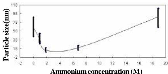
Figure 8: Effect of the initial ammonia concentration on the average and range of nickel particles size
