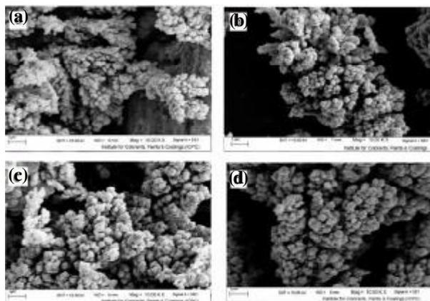
Figure 5: SEM images of nickel nanopowder samples which were synthesized at temperatures of 0°C (a), 25°C (b), 45°C (c) and 100°C (d)
