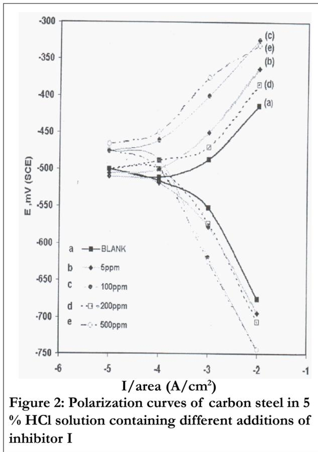
Figure 2: Polarization curves of carbon steel in 5 % HCl solution containing different additions of inhibitor I
