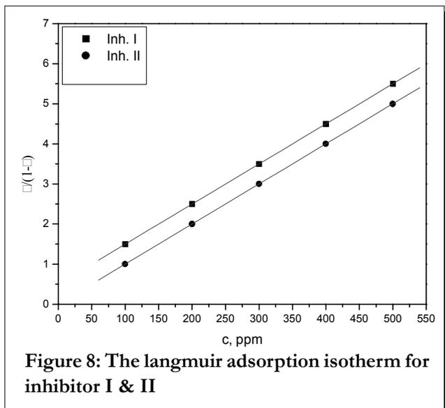
Figure 8: The langmuir adsorption isotherm for inhibitor I & II
