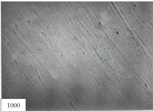
Figure 12: (X-1000) after 1hr immersion in 5 % HCl containing 500 ppm dose of inhibitor II sample D.
