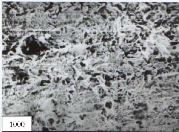
Figure 10: (X-1000) after 1hr immersion in 5 % HCl solution sample B
