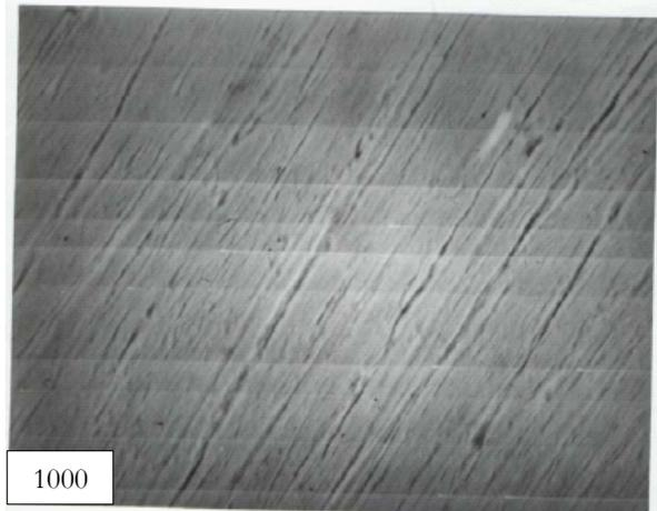
Figure 11: (X-1000) after 1hr immersion in 5% HCl containing 500 ppm dose of inhibitor I sample C.
