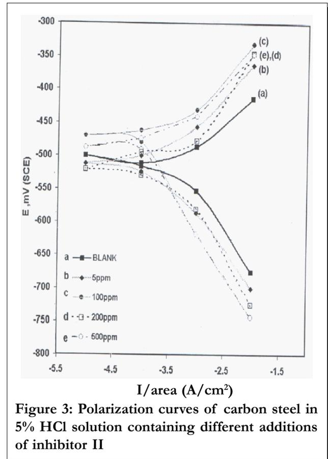
Figure 3: Polarization curves of carbon steel in 5% HCl solution containing different additions of inhibitor II
