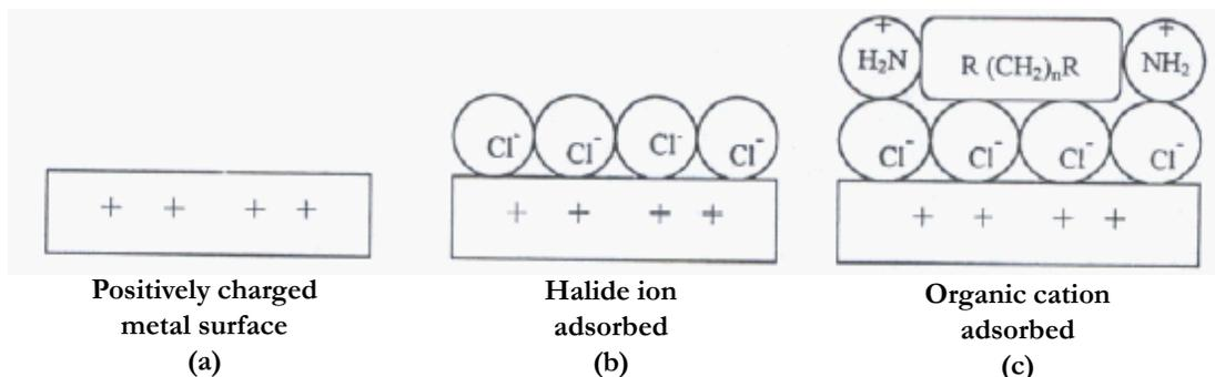
Figure 13: Schematic adsorption mechanism positively charged metal surface in presence of 5 % HCl solution.
