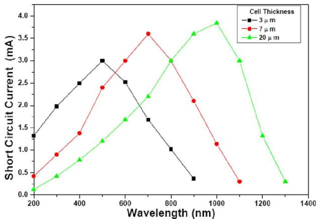
Figure 4 : Spectral response for different cell thickness
