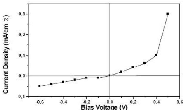
Figure 1 : Current -voltage characteristic in dark
