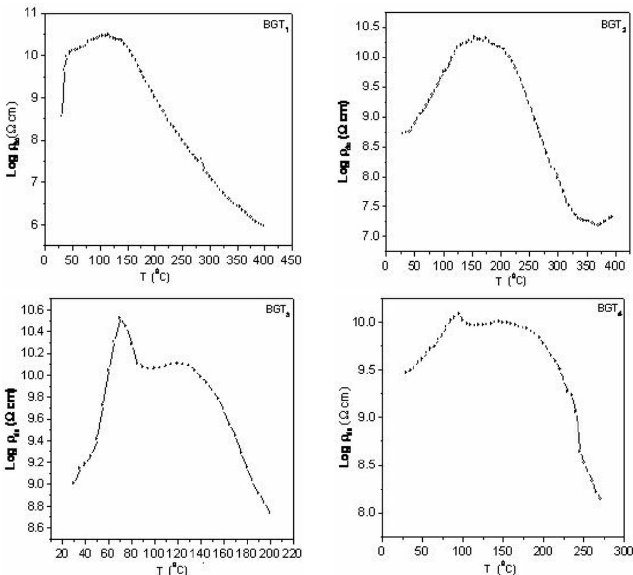
Figure 1 : Temperature dependence of resistivity behaviour of BGT ceramics
