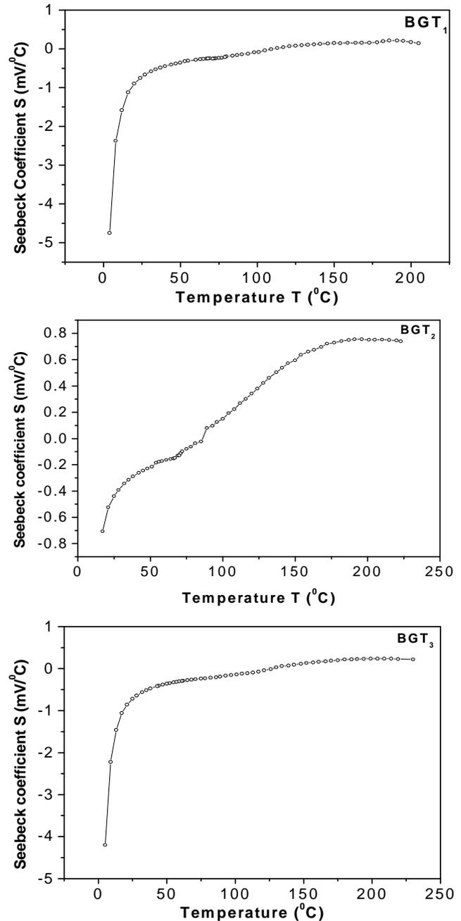
Figure 2 : Thermoelectric characteristics of BGT ceramics
