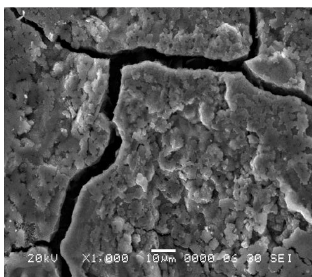
Figure 9 : Images of iron rod photographed under SEM after soaking them in the simulated acid rain sample of pH 3
