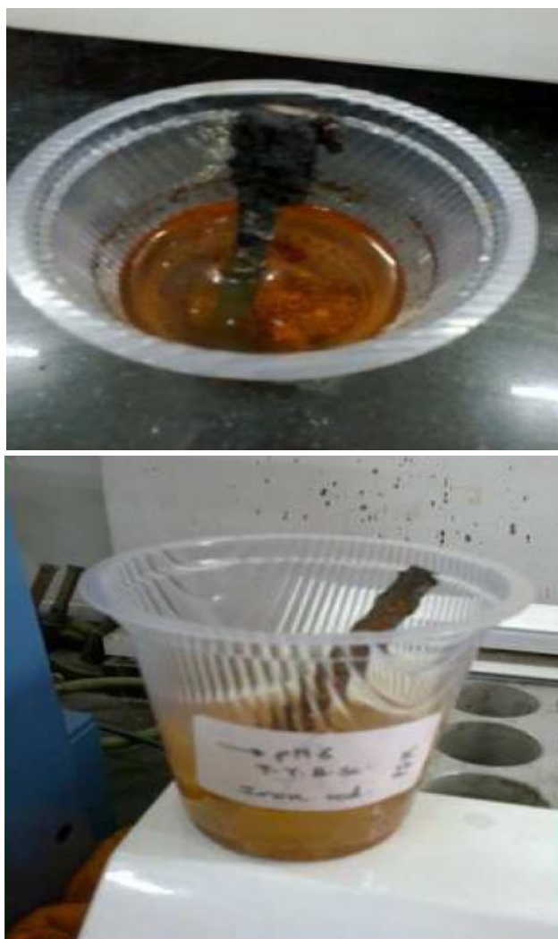
Figure 7 : Iron rod in pH 3 (Left) and pH 6 (Right)
