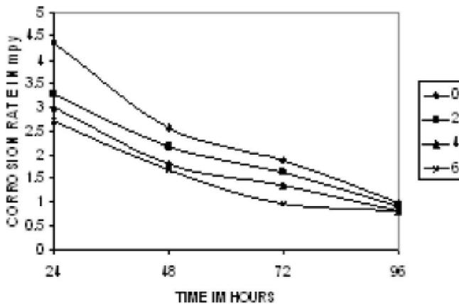
Figure 2 : Weight loss corrosion in 0.35% sodium chloride solution
