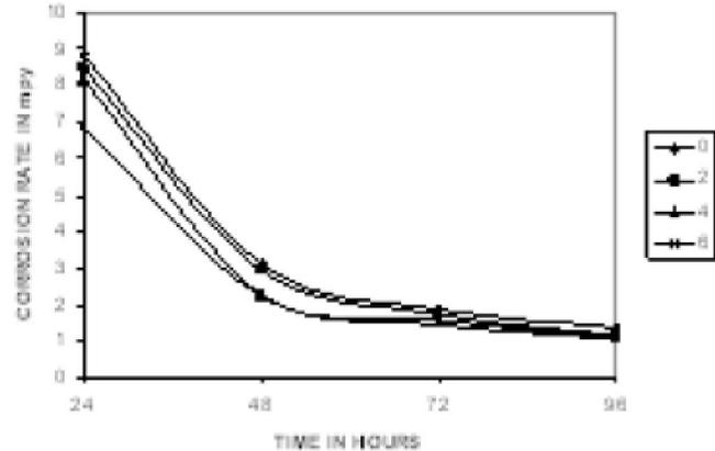
Figure 3 : Weight loss corrosion in 3.5% sodium chloride solution
