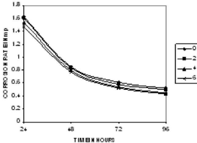
Figure 1 : Weight loss corrosion in 0.035% sodium chloride solution
