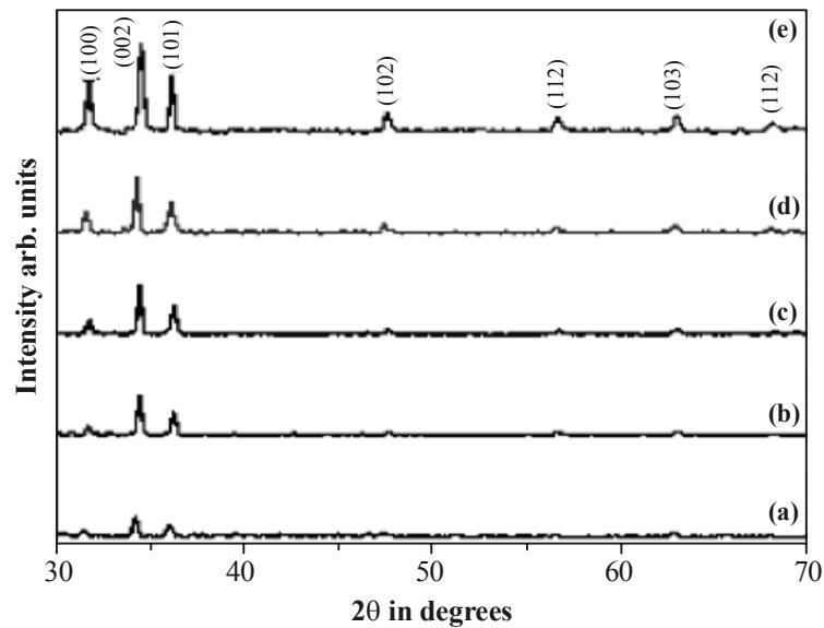
**Fig. 1: The effect of number of dipping on the XRD patterns of ZnO thin films**
