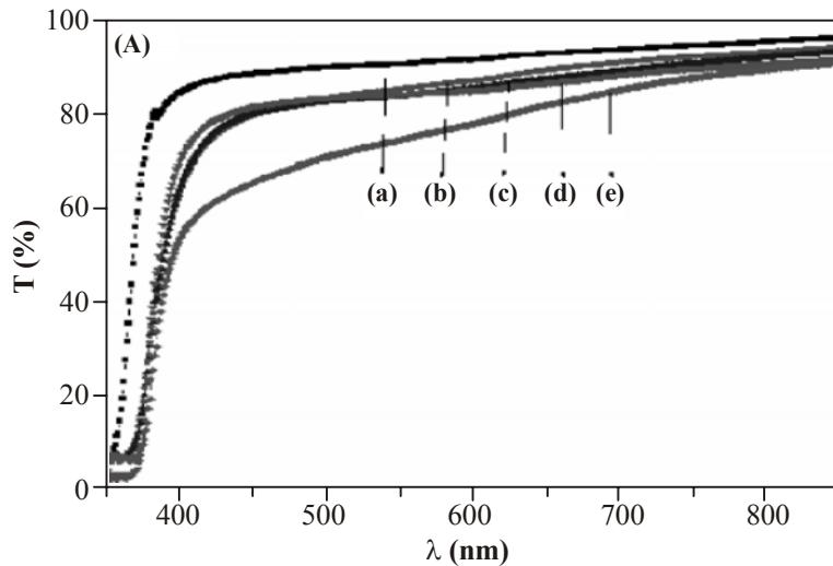
**Fig. 4: Optical transmittance spectra of ZnO thin films prepared from different dipping
