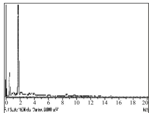
Fig. 3(f): EDAX spectrum of a ZnO film grown at 125 dipping
