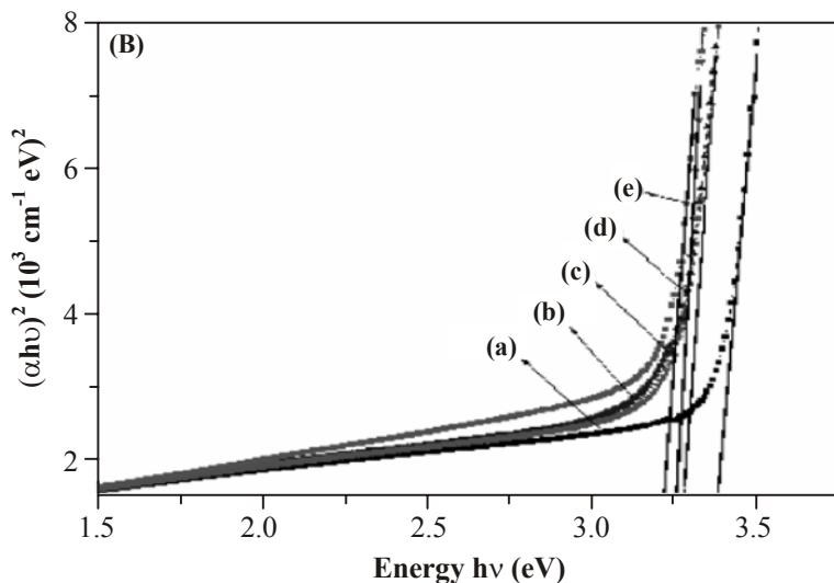
**Fig. 5: Plot of  $(hv)$  vs  $(hva)^2$  of ZnO thin films prepared from different number of dipping (a) 50, (b) 75, (c) 100, (d) 125 and (e) 150**
