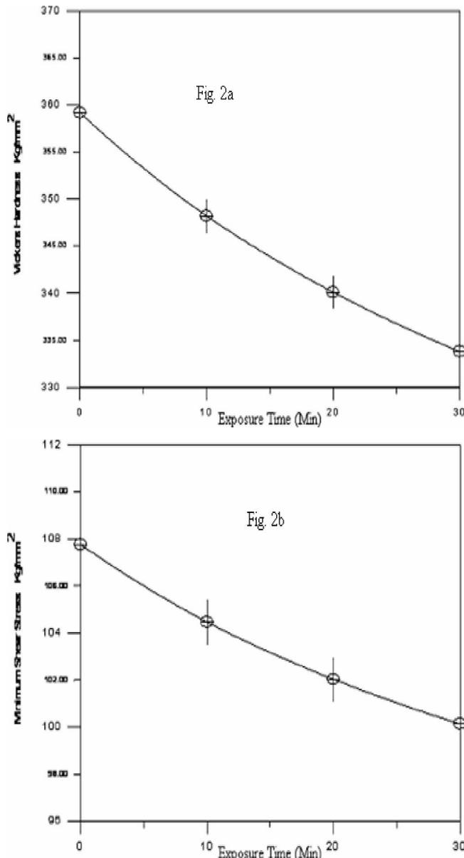
Figure 2 : Vickers hardness and minimum shear stress of Protechno® -N alloy before and after exposure to MRI
