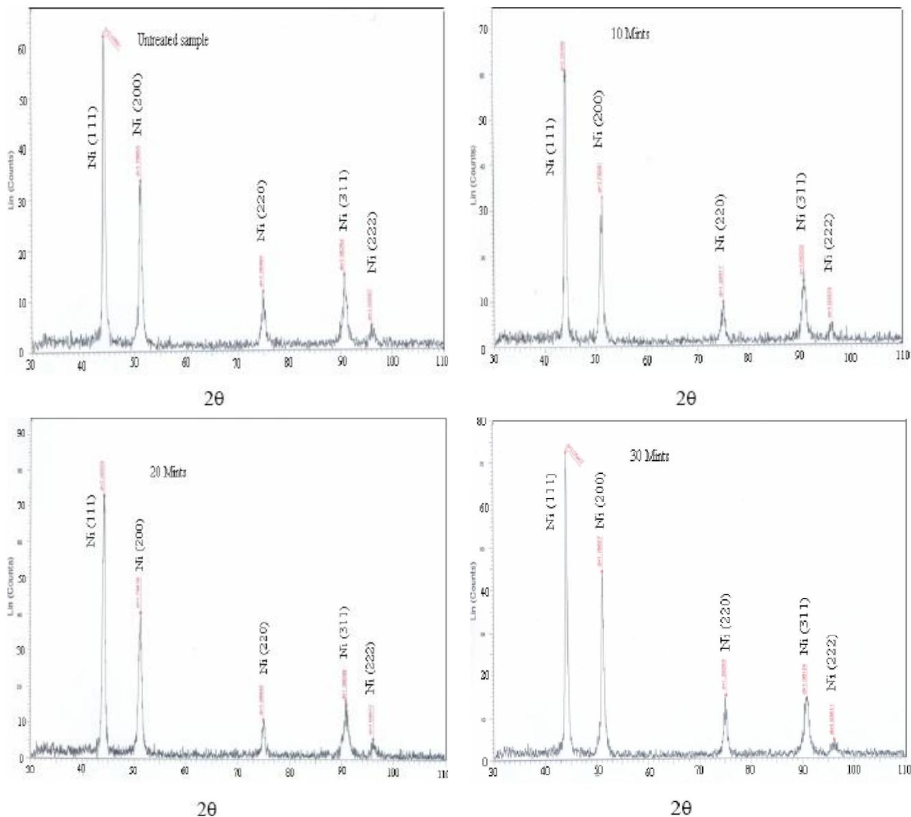
**Figure 1 : x-ray diffraction patterns of Protechno® -N alloy before and after exposure to MRI**
