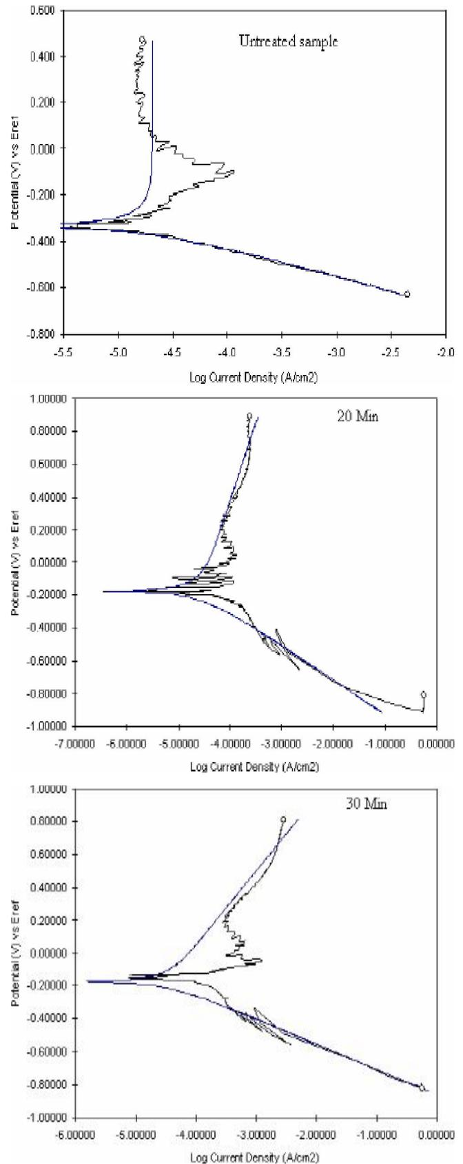
Figure 4 : electrochemical polarization curves for Protechno® -N alloy before and after exposure to MRI
