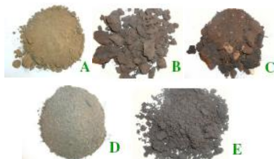
Figure 1: Colour and texture of the soil samples- A: Control sample B: Long duration impact sample C: Short duration impact sample, D: Short duration with amendment sample E: Instant impact sample
