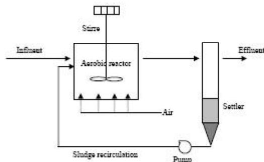
Figure 1: Schematic diagram of the experimental set-up
