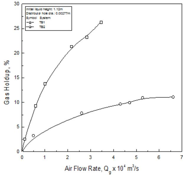
FIG. 3. Effect of the column diameter on holdup.
