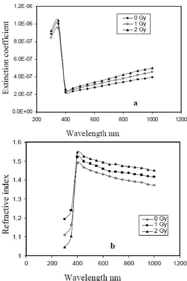
Figure 3 : The variation of a)  $k$  & b)  $n$  with (Wavelength) of doped PMMA films at different doses irradiation.
