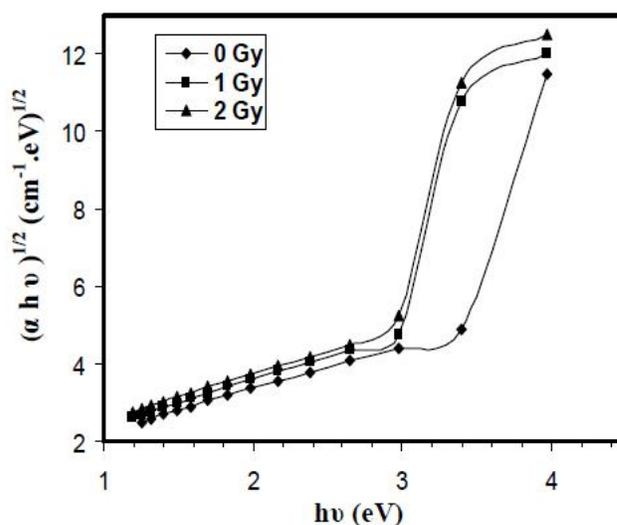
Figure 2 : The variation of  $(\alpha h\nu)^{1/2}$  with  $(h\nu)$  of doped PMMA films at different doses irradiation.
