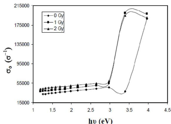
**Figure 5 :** The variation optical conductivity  $\sigma_0$  with  $(h\nu)$  of doped PMMA films at different doses irradiation.
