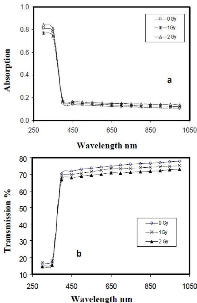
Figure 1 : The variation of a) Absorption and b) Transmission spectra with (Wavelength) of doped PMMA films at different doses irradiation.
