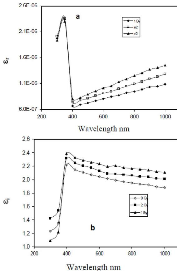
Figure 4 : The variation of a)  $\epsilon_i$ , b)  $\epsilon_r$  with Wavelength (nm) of doped PMMA films at different doses irradiation.
