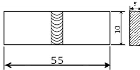
**Fig. 5: Dimensions of impact test specimen**
