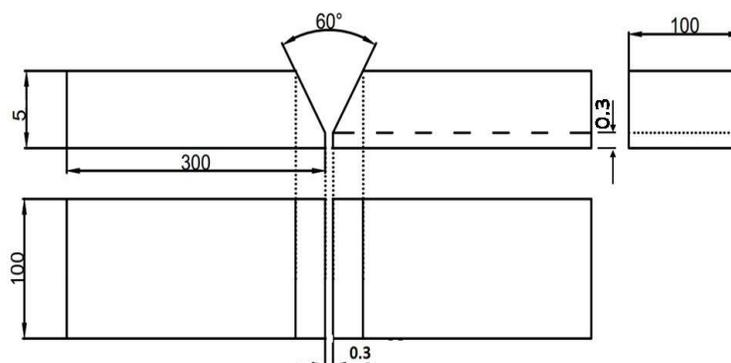
**Fig. 3: Dimensions of stainless steel and mild steel plates for welding**
