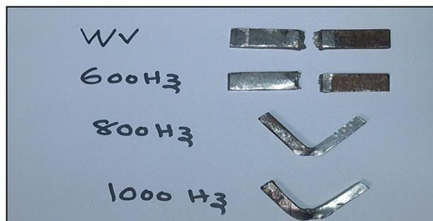
**Fig. 7: Specimens after impact testing**
