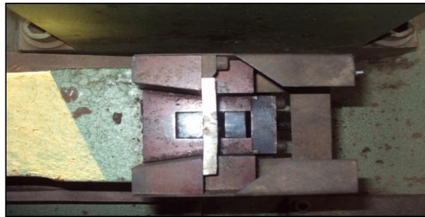
**Fig. 6: Specimen ready for impact test**
