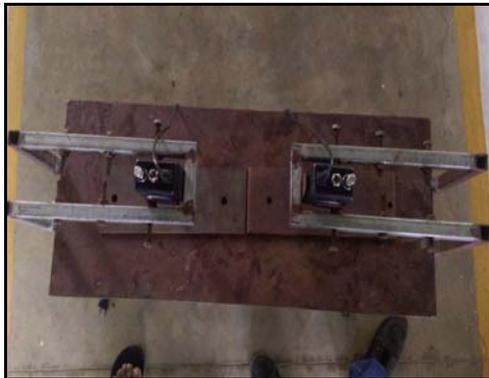
**Fig. 2: Top view of vibratory welding setup with specimens ready for welding**
