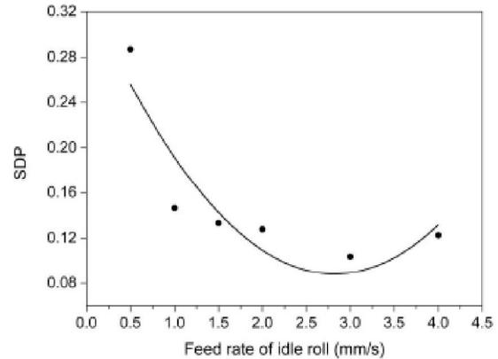
Figure 4 : Effect of feed rate of roll on  $SDP$
