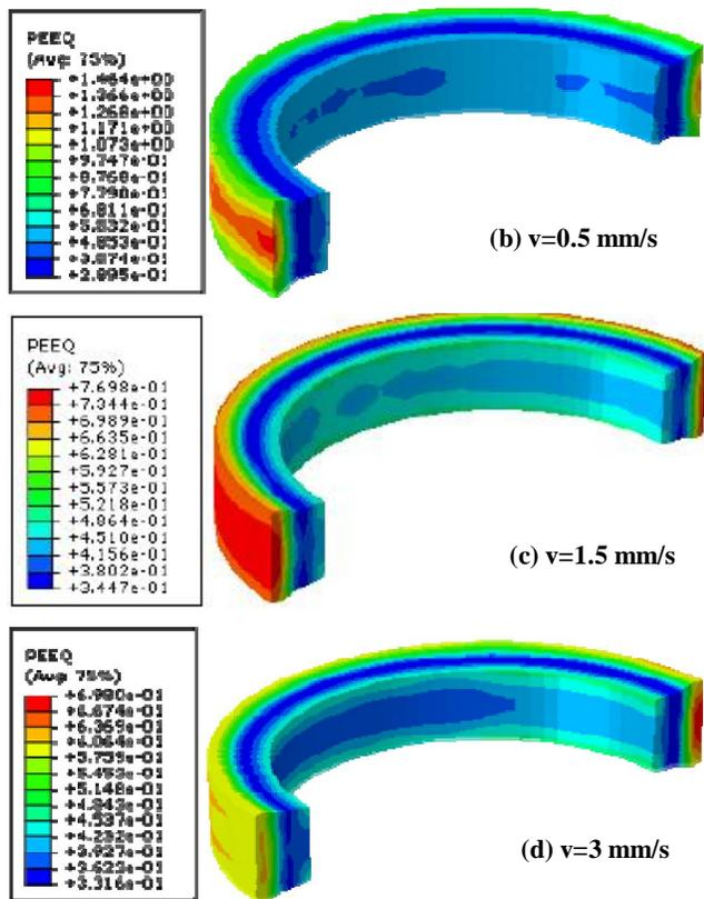
Figure 5 : Equivalent strain distribution of rolled ring
