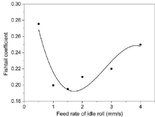
Figure 8 : Effect of  $v$  on fishtail coefficient
