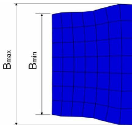
Figure 3 : The axial spread of the rolled ring
