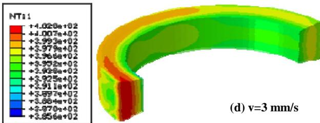
Figure 7 : Temperature distribution of rolled ring
