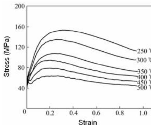
Figure 2 : The true stress-strain curves model for hot ring of AZ31 magnesium alloy
