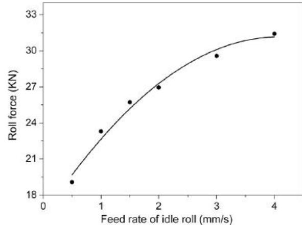
Figure 9 : Effect of  $v$  on roll force
