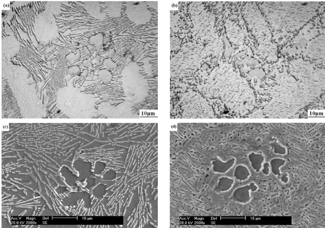
Figure 2 : Microstructures of the as-cast and aged  $\text{Al}_{0.5}\text{B}_{0.2}\text{CoCrFeNi}$  alloys: (a) as-cast (OM), (b) aged at 1000 °C (OM),
