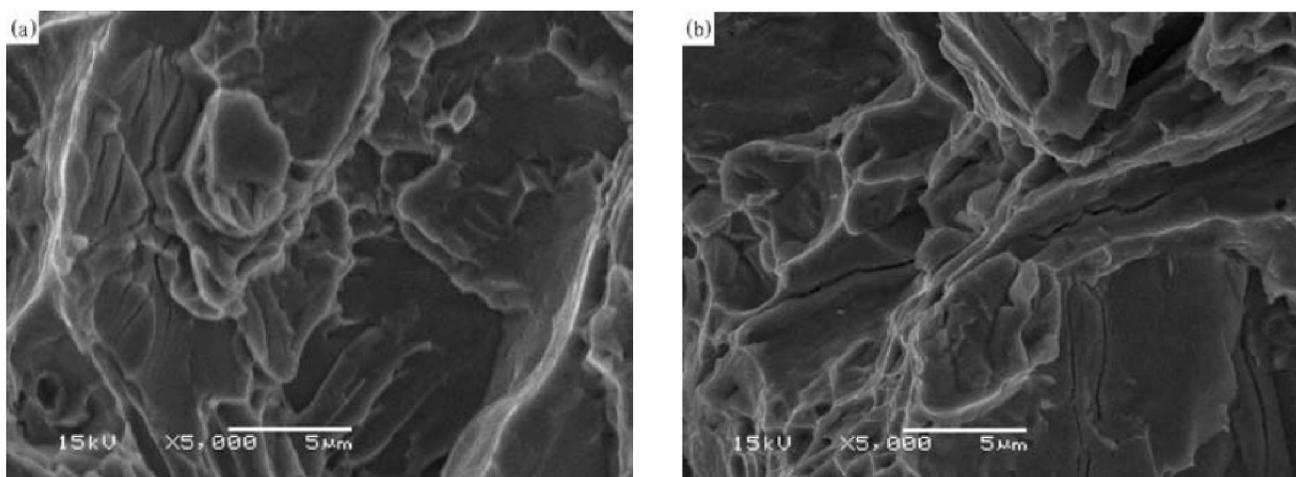
Figure 4 : SEM of tensile fracture surface of the as-cast and aged  $\text{Al}_{0.5}\text{CoCrFeNiB}_{0.2}$  alloys: (a) as-cast, (b) aged at 1000°C
