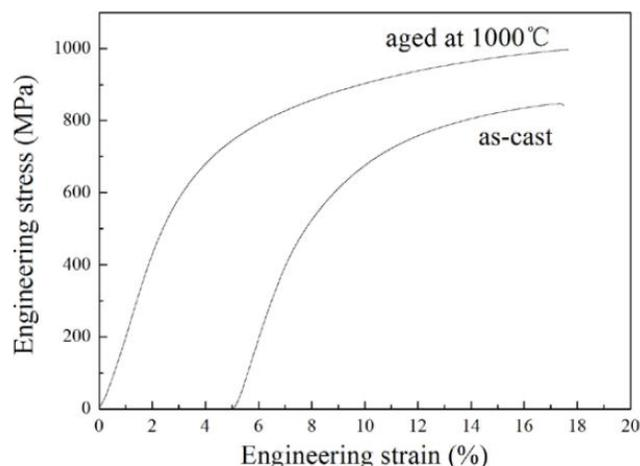
Figure 3 : Room-temperature tensile curves of the as-cast and aged  $\text{Al}_{0.5}\text{CoCrFeNiB}_{0.2}$  alloys
