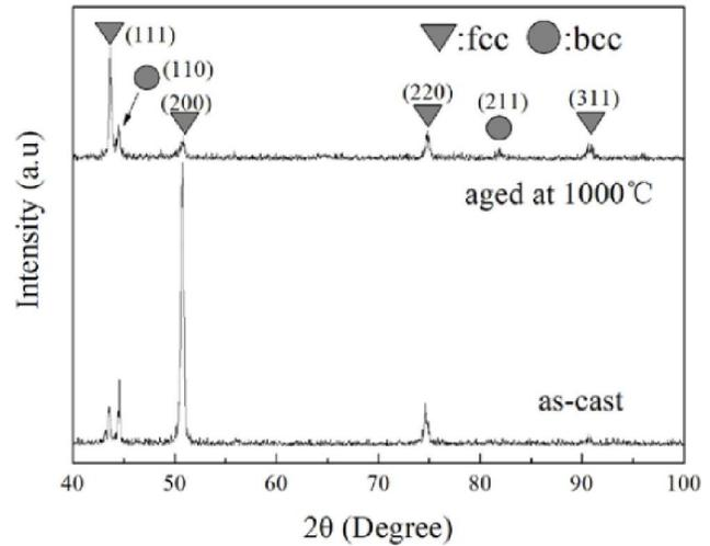
Figure 1 : XRD patterns of the as-cast and aged  $\text{Al}_{0.5}\text{CoCrFeNiB}_{0.2}$  alloys
