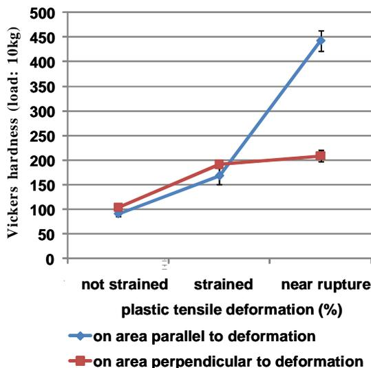
Figure 2 : Evolution of the Vickers hardness with the state of strain for the two orientations (load 10kg)
