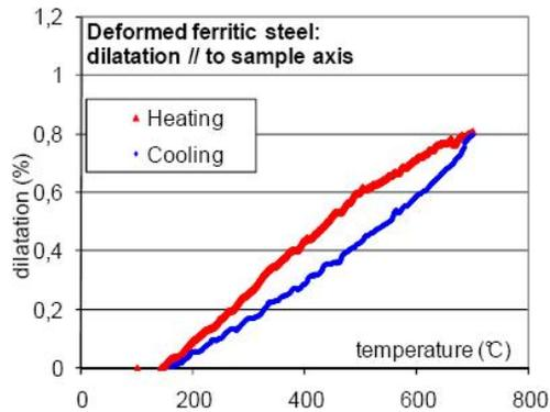
Figure 3b : Dilatometry curves of the strained state for the two orientations
