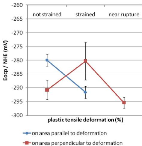
Figure 4a : Evolution of the open circuit potential with the state of strain for the two orientations
