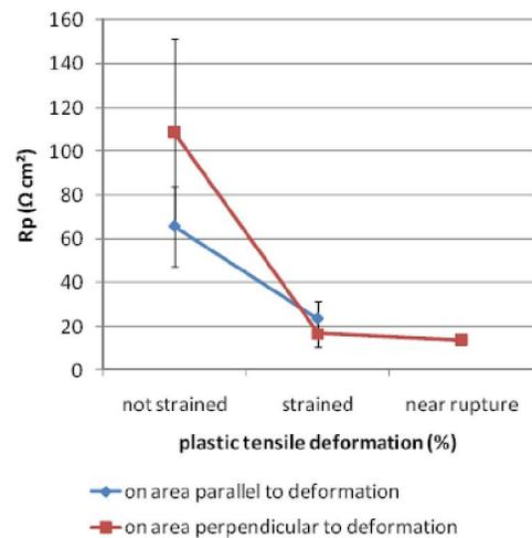
Figure 4b : Evolution of the polarization resistance with the state of strain for the two orientations
