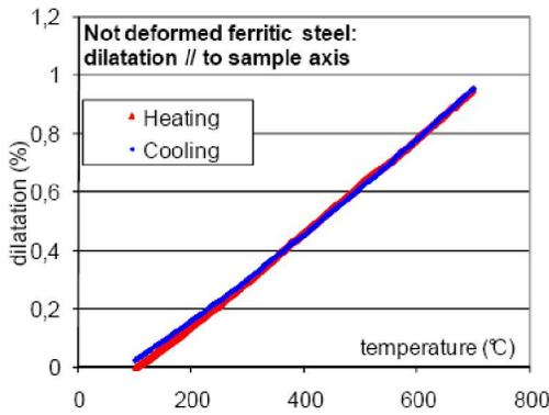
Figure 3a : Dilatometry curves of the not strained state for the two orientations
