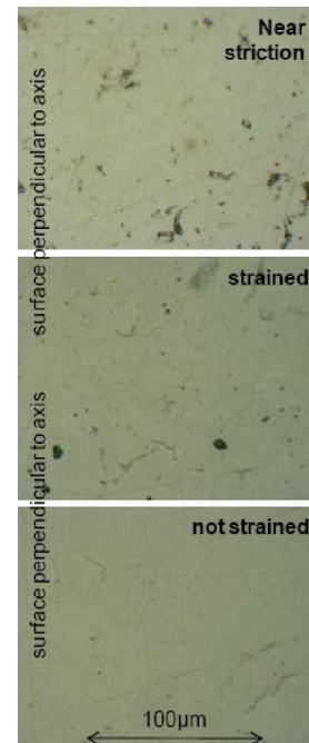
**Figure 1b : Microstructures of the steel for the three states of deformation and for the orientation perpendicular to the strain direction (optical micrograph after Nital4-etching)**
