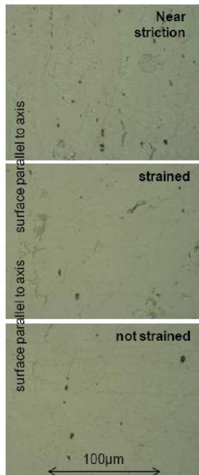
**Figure 1a : Microstructures of the steel for the three states of deformation and for the orientation parallel to the strain direction (optical micrograph after Nital4-etching)**
