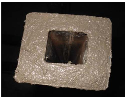
**Fig. 3: Concrete filled CFDST specimen**
