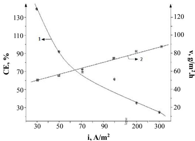
**Fig. 1:** Effect of current density of the zinc electrode on current efficiency (1) and the dissolution rate of the metal (2) ( $\text{CH}_3\text{COOH} = 100 \text{ g/L}$ ,  $\tau = 0,5 \text{ h}$ ,  $t = 20^\circ\text{C}$ )
