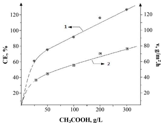
**Fig. 2: Effect of concentration of acetic acid on current efficiency (1) and the dissolution rate of the metal (2) ( $i = 50 \text{ A/m}^2$ ;  $\tau = 0,5 \text{ h}$ ;  $t = 25^\circ\text{C}$ )**
