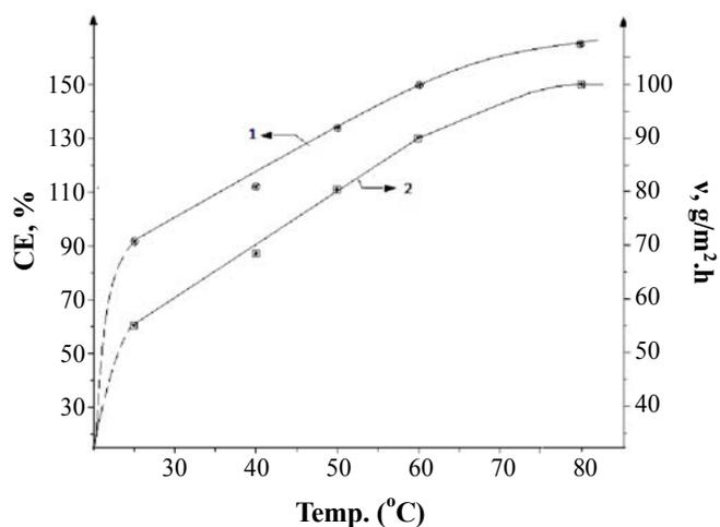
**Fig. 4: Effect of temperature on the current efficiency (1) and the dissolution rate of zinc (2) ( $C_{\text{CH}_3\text{COOH}} = 100 \text{ g/L}$ ;  $i_{\text{Zn}} = 50 \text{ A/m}^2$ ;  $\tau = 0,5 \text{ h}$ )**
