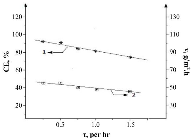
**Fig. 3: Effect of the duration of the electrolysis on current efficiency (1) and the dissolution rate of zinc (2) ( $\text{CH}_3\text{COOH} = 100 \text{ g/L}$ ;  $i = 50 \text{ A/m}^2$ ;  $t = 25^\circ\text{C}$ )**
