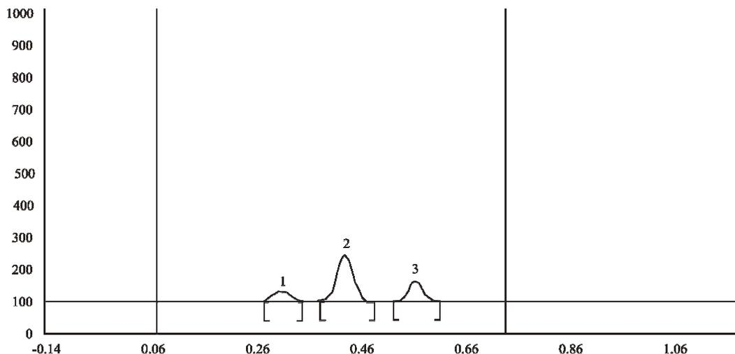
**Fig. 4: Densitogram of acid (1N HCl, reflux for 2 h, temp 70°C) treated drug; peak 1 (degraded) ( $R_f : 0.35$ ), peak 2 (degraded) ( $R_f : 0.47$ ), peak 3 (Standard) ( $R_f : 0.625$ )**
