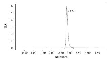
Fig. 2: Chromatograph of standard temozolomide preparation
