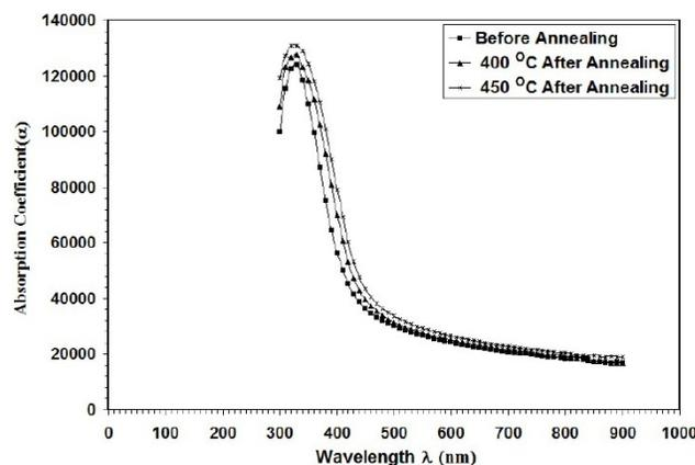
Figure 1 : Absorption coefficient versus wavelength for CdO:6%Mg films
