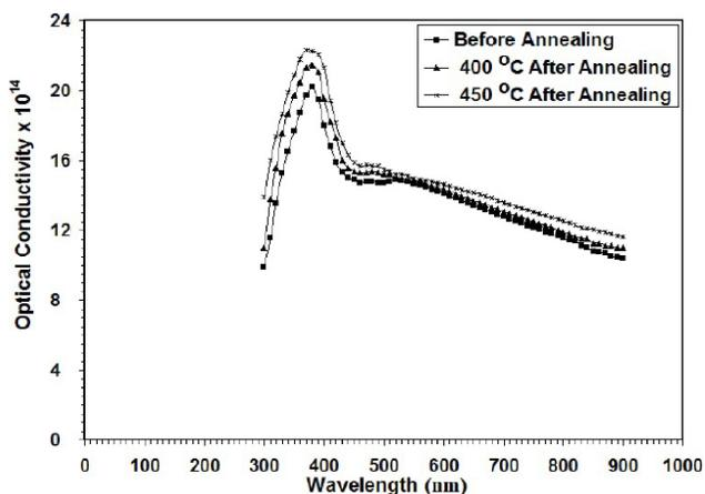
Figure 5 : Optical conductivity versus wavelength for CdO:6%Mg films
