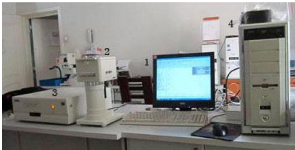
1. Measuring software, 2. Measuring chamber, 3. Signal analyzer host, 4. Data processing system
