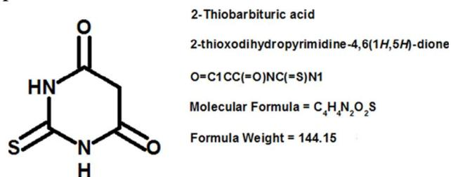
**Figure 1 : Structure and properties of 2-thiobarbituric acid. The molecular structure, common name, SMILES notation, and formula presented here for the sedative/hypnotic compound 2-thiobarbituric acid.**
