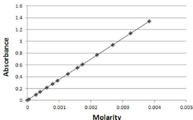
**Figure 3 :** Standard curve of assay by spectrophotometer. The standard curve utilized in this study ranged from 0.00004570 molar to 0.003830 molar (a 84x wide range in molar concentration values).
