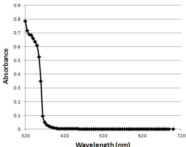
**Figure 2 :** Absorbance spectrum of 2-thiobarbituric acid from 320 nm to 700 nm obtained in glass cuvettes and 95% ethanol with 5% water.
