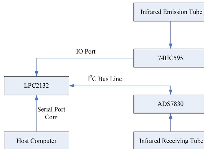
**Figure 5 : Realizing principle of infrared touch screen**
