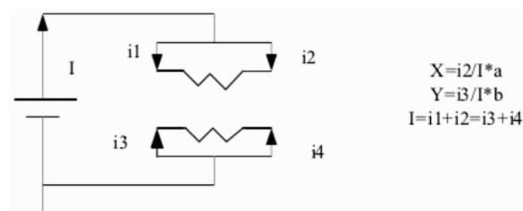
Figure 1 : Principle of capacitive touch screen
