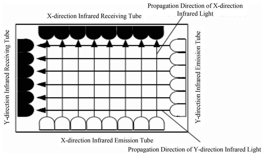
**Figure 4 : Structure of infrared touch screen**
