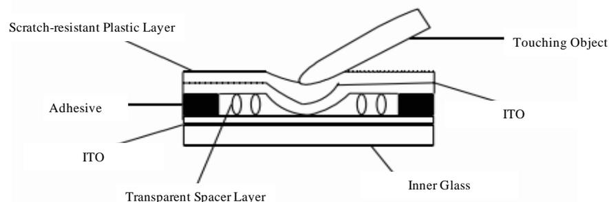
Figure 2 : Structure of resistive touch screen
