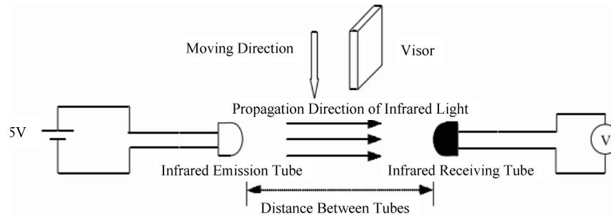
**Figure 6 : Structure of testing device**
