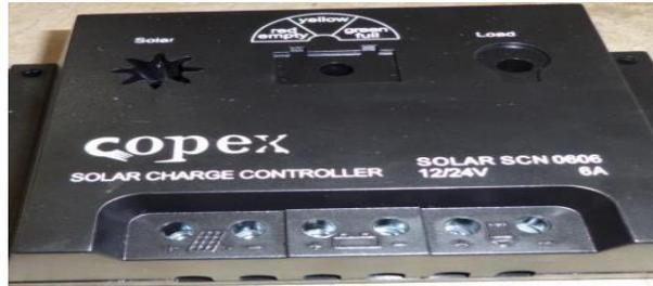
FIG. 7. Solar charge controller.
