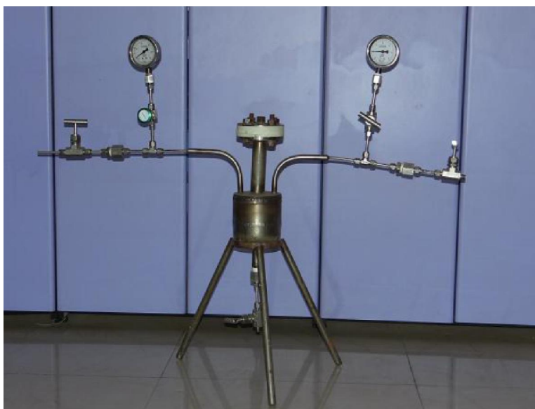
Figure 1 : Pressure vessel for storage of hydrogen as uranium hydride
