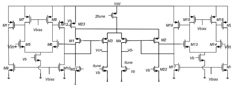
**Fig. 2: Transconductance amplifier**
