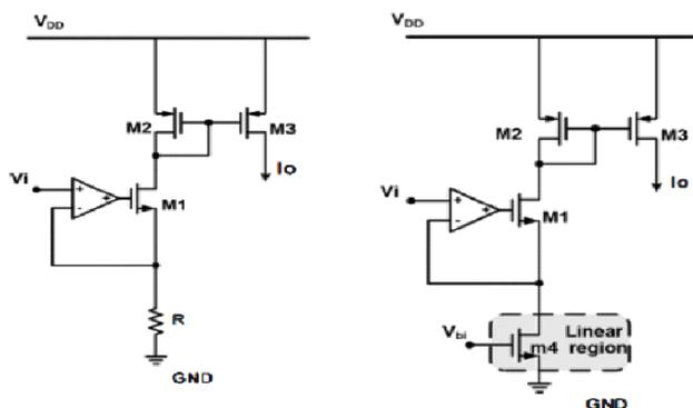
**Fig. 1: Transconductor amplifier with (a) Resistor (b) MOSFET**
