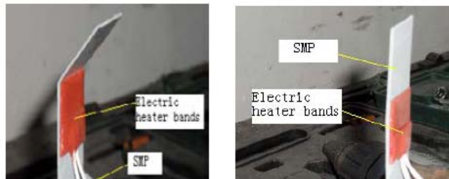
Figure 3: Shape memory polymer before and after electrothermal stimulation
