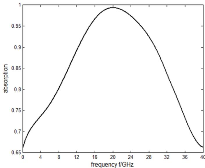
**FIG. 2. The absorption properties of the vertical incident electromagnetic wave.**
