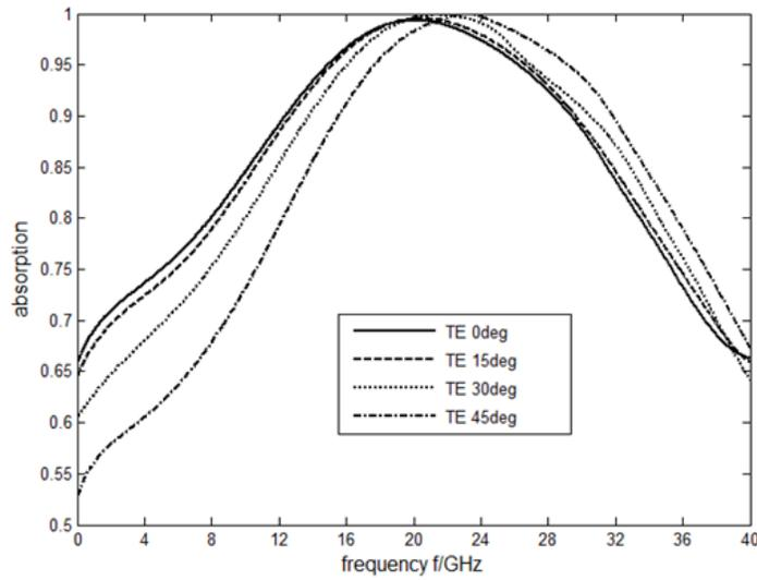
FIG. 3. The absorption properties for transverse electric (TE) polarization.
