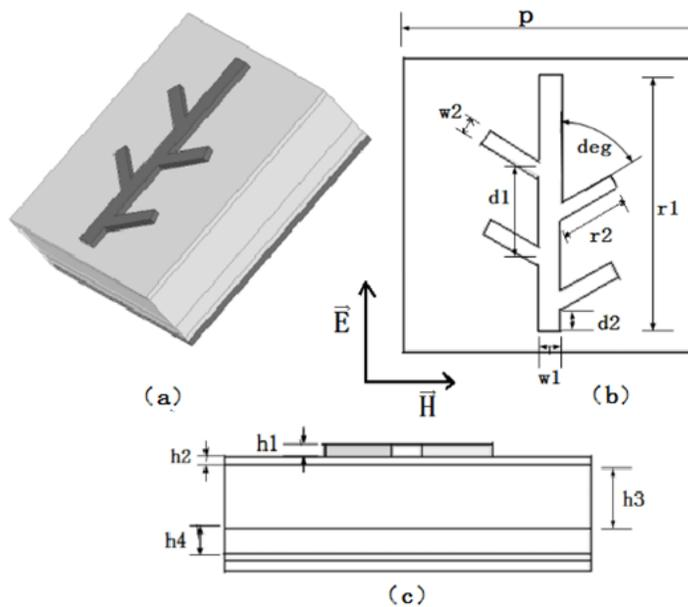
**FIG. 1. (a) Schematic structure of the designed metamaterial absorber (b) The front and (c) oblique view of the unit cell.**
