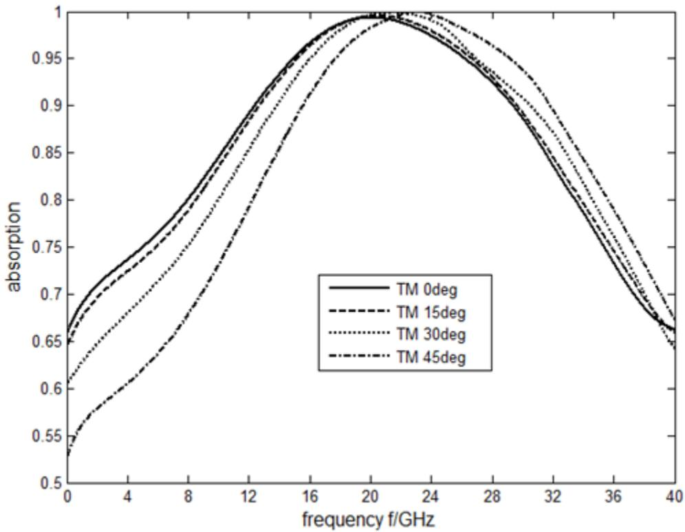
FIG 4. The absorption properties for transverse magnetic (TM) polarization.
