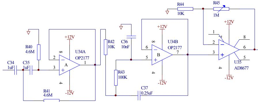
**Figure 4 : Band-pass filter and main amplifier circuit diagram**
