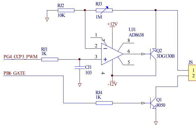
**Figure 6: Stimulator pulse generator circuit**
