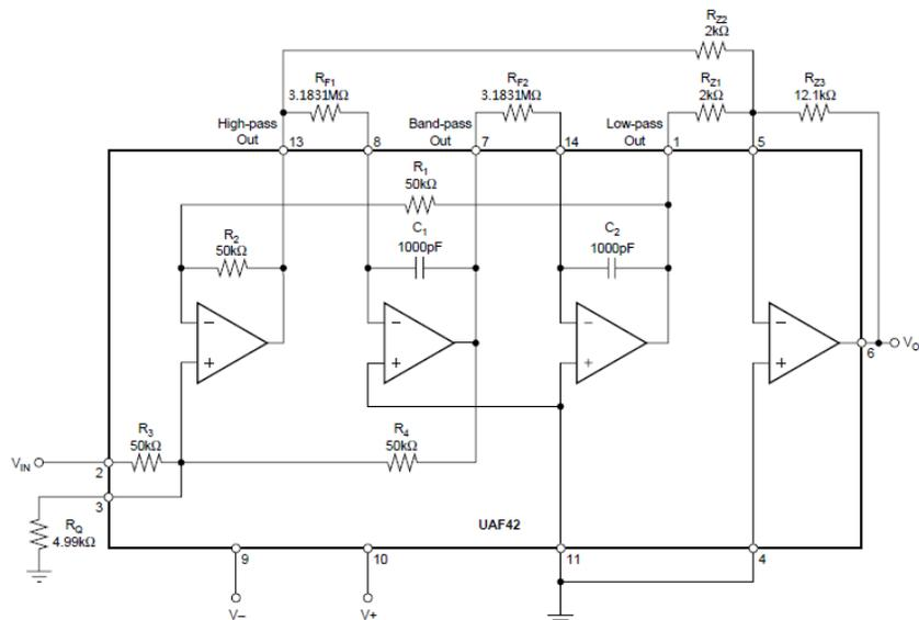
**Figure 5 : UAF42 configured as a 50HZ notch filter**
