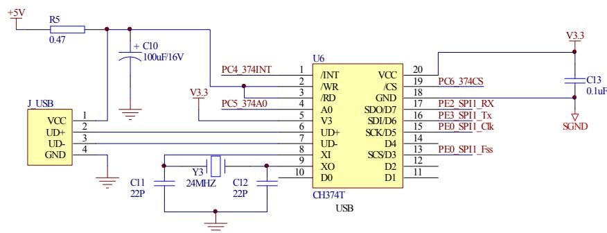
**Figure 8: CH374 interface circuit**
