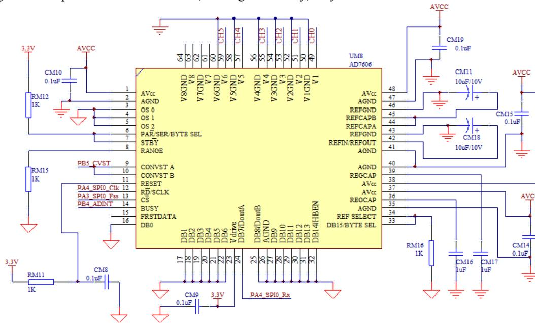
Figure 7: AD7606 interface circuit
