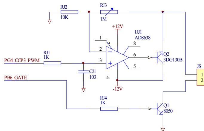
**Figure 6: Stimulator pulse generator circuit**
