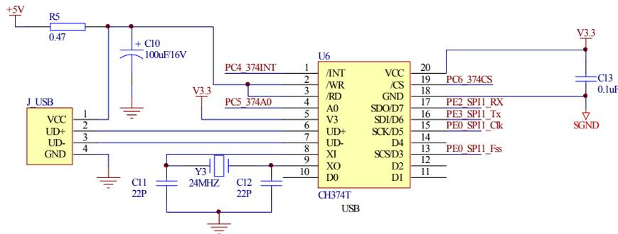
Figure 8: CH374 interface circuit
