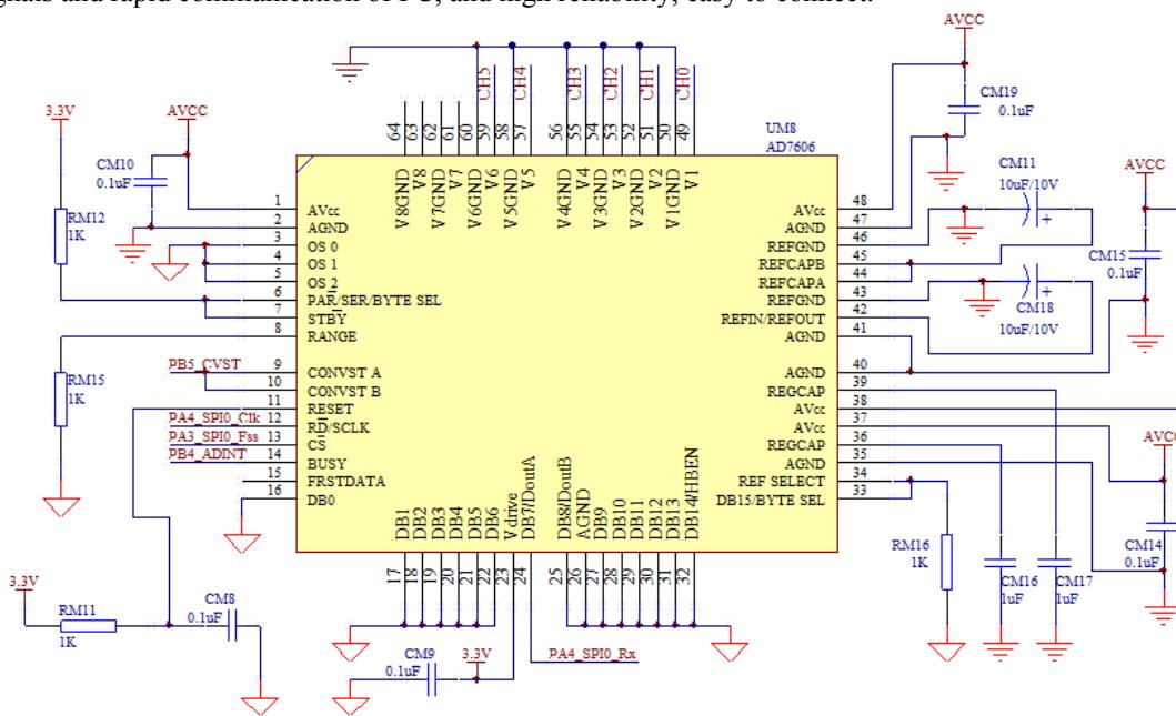
**Figure 7: AD7606 interface circuit**
