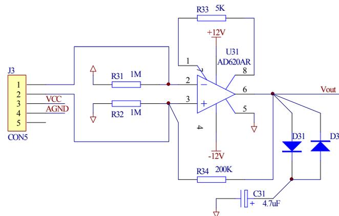
**Figure 3: Preamplifier circuit diagram**
