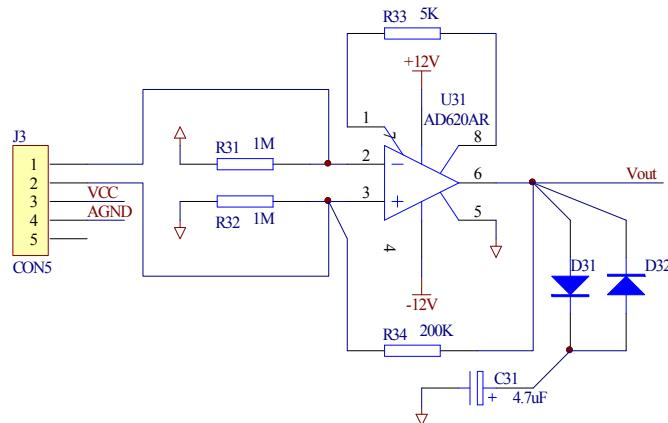
**Figure 3: Preamplifier circuit diagram**
