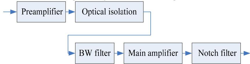
**Figure 2 : Pre-processing circuit diagram**
