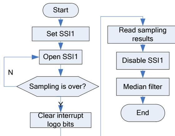
**Figure 10: Flow chart of data acquisition of SSI interrupt service program**
