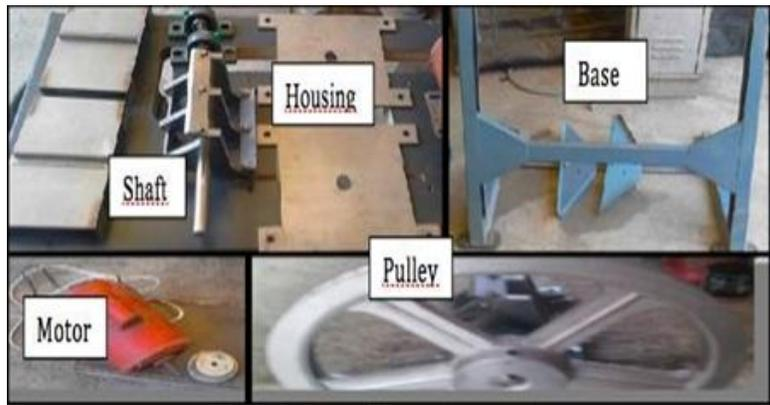
**FIG. 6.** Pieces of the crushing machine
