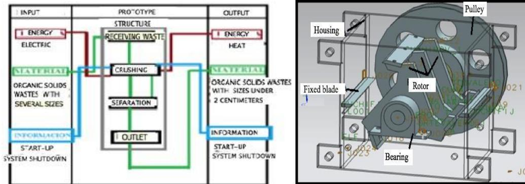
**FIG. 4.** Service functions and their interrelationships [8]. **FIG. 5.** 3D model of crushing machine
