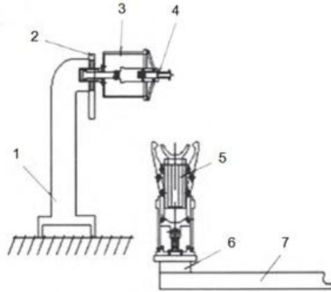
(1- fixture strains,2-sliding caliper,3-cutter gripper,4-cutter,5-mechanical hand,6-mechanical hand rotating seat,7-fixed mount)
