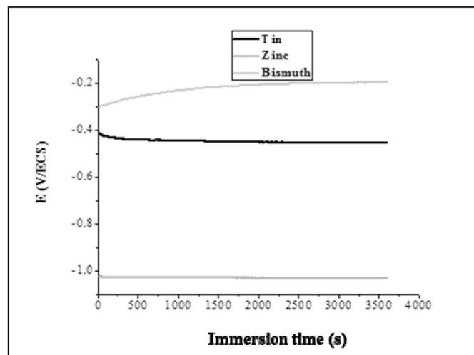
Figure 2 : OCP curves of pure tin, zinc and bismuth after an hour of immersion in NaCl 3% solution
