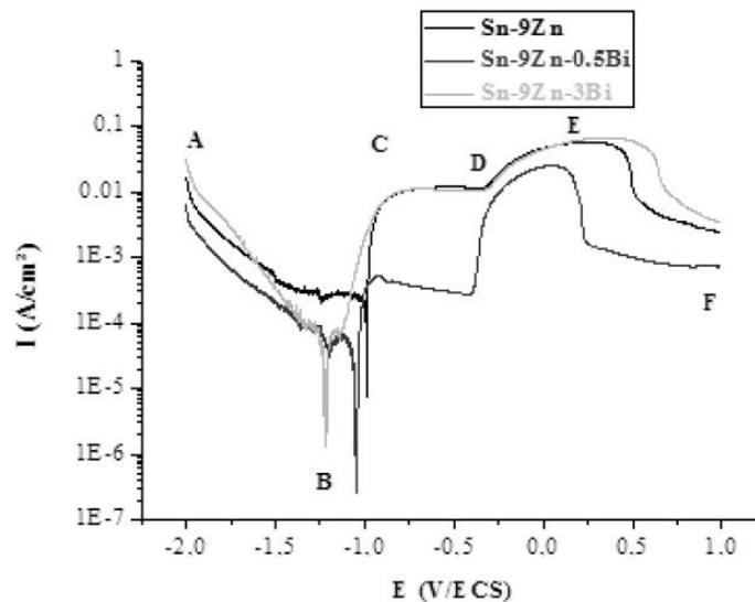
Figure 3 : Polarization curves of the studied solder alloys in NaCl 3 wt.% solution
