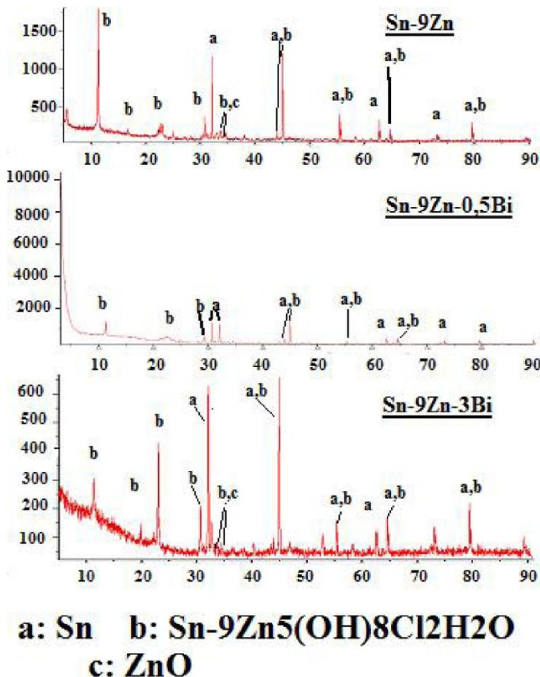
Figure 5 : XRD spectra of our alloys after a week of immersion in NaCl 3 wt.% solution
