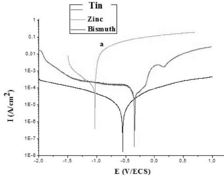
Figure 4 : Polarization curves of the studied solder alloys in NaCl 3 wt.% solution
