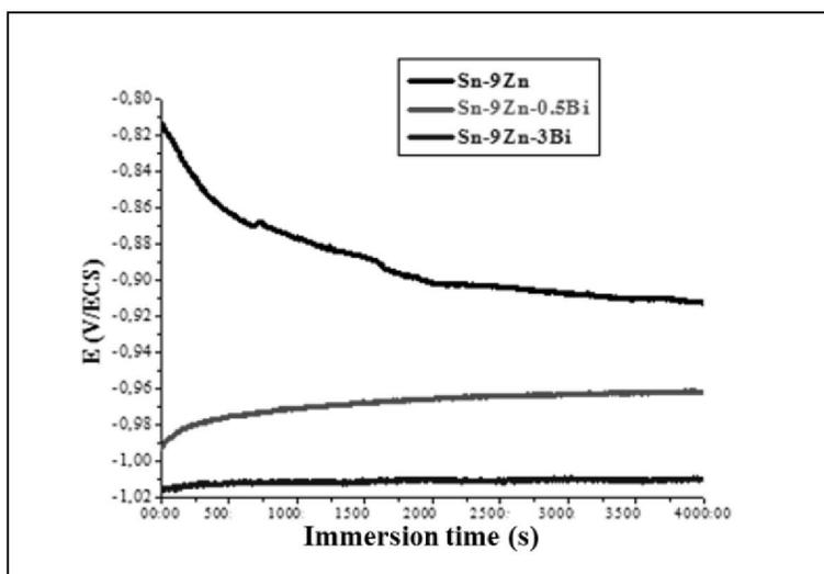
Figure 1 : OCP curves of the three studied alloys after an hour of immersion in NaCl 3% solution
