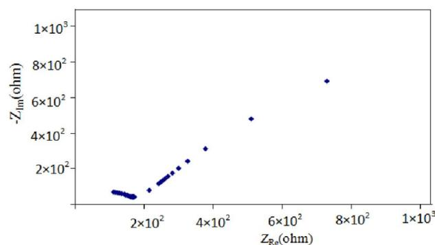
Figure 5 : AC impedance spectrum of P(VIM-co-BuMA-HBF<sub>4</sub>) at 30°C
