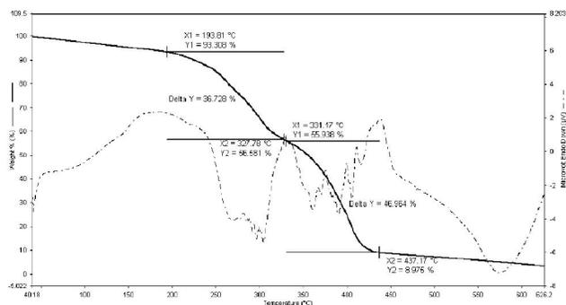
Figure 3(b) : TGA curve of P(VIM-co-BuMA-HBF<sub>4</sub>)
