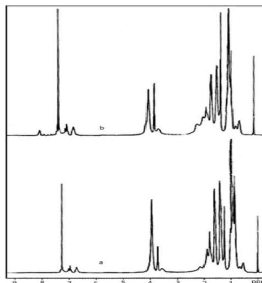
Figure 2 : <sup>1</sup>H NMR spectra of (a) P(VIM-co-BuMA) (b) P(VIM-co-BuMA-HBF<sub>4</sub>)
