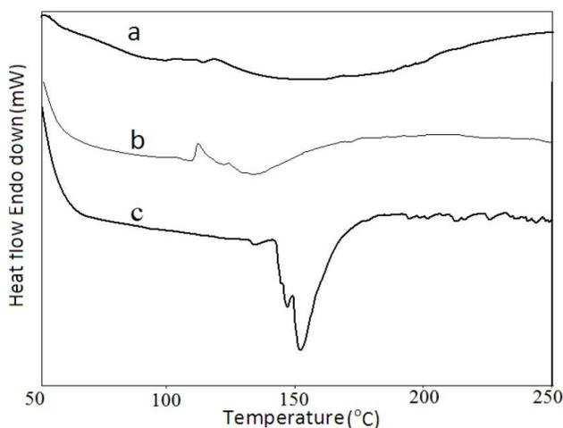
Figure 4 : DSC curves of (a) PVIM (b) P(VIM-co-BuMA) (c) P(VIM-co-BuMA-HBF<sub>4</sub>)
