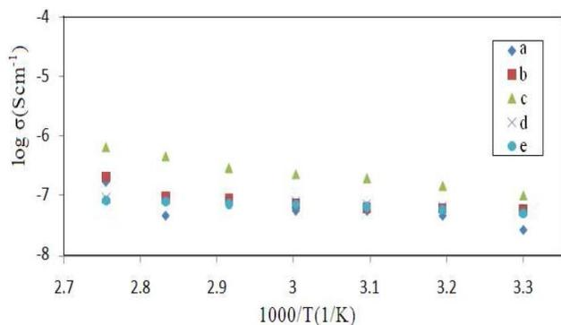
Figure 6(a) : Plot of  $\log \sigma$  vs.  $1/T$  of P(VIM-co-BuMA)
