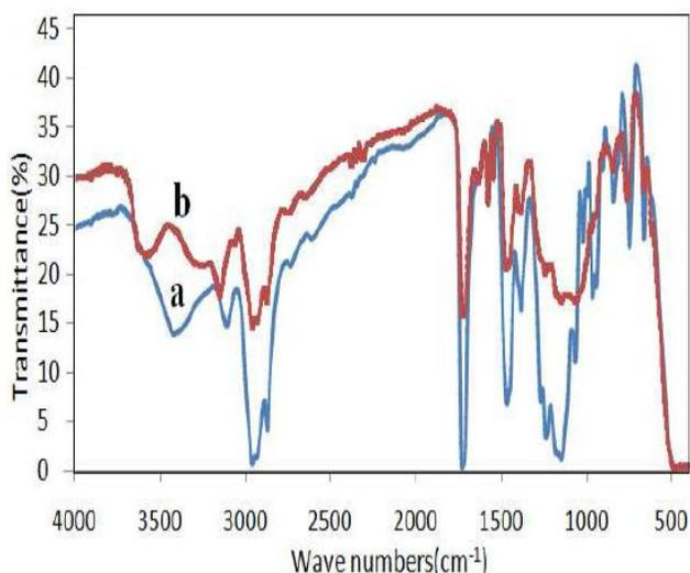
Figure 1 : IR spectra of (a) P(VIM-co-BuMA) (b) P(VIM-co-BuMA-HBF<sub>4</sub>)
