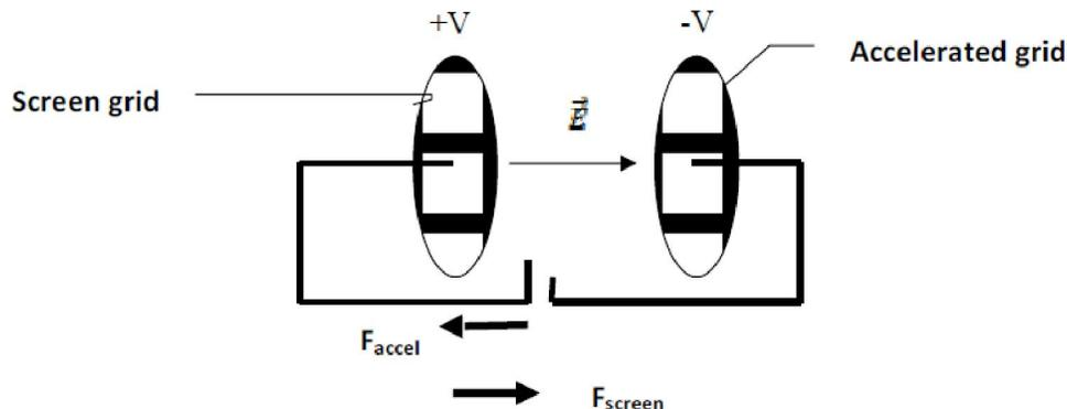
Figure 3 : Forces on a two-grid acceleration system
