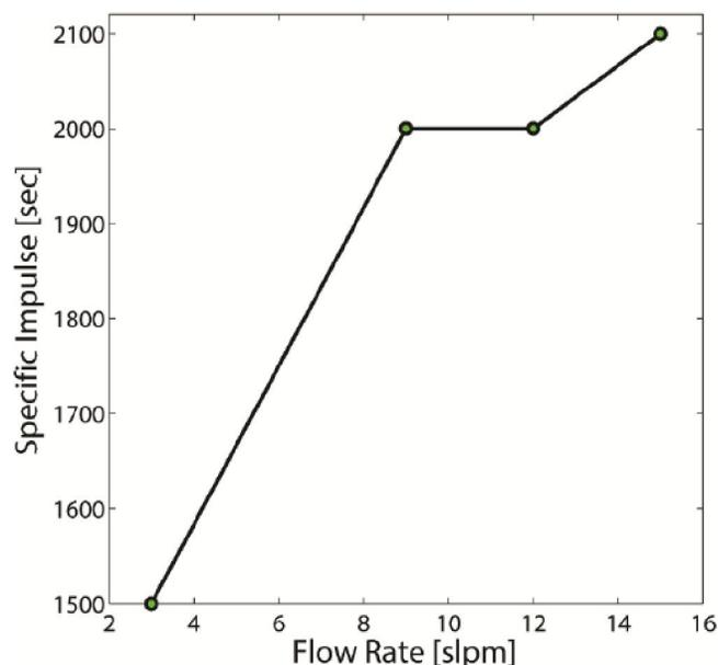
Figure 8 : Variation of the specific impulse with gas flow rate at 3 MHz
