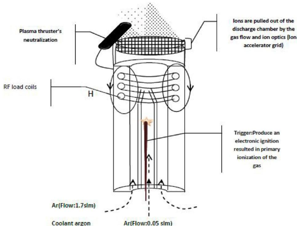
Figure 2 : A simplified schematic of the plasma thruster
