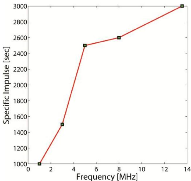
Figure 7 : Variation of the specific impulse versus frequency
