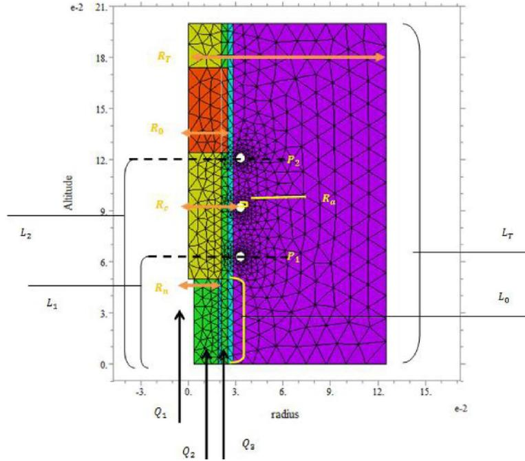
Figure 4 : Torch geometry; RF current is applied to two ends  $P_1$  and  $P_2$ . Argon gas flows into the inlet region of the torch tube with different flow rates  $Q_1$ ,  $Q_2$ , and  $Q_3$ . Plasma is generated in the coil region with radius  $R_n$  which is less than  $R_0$ .
