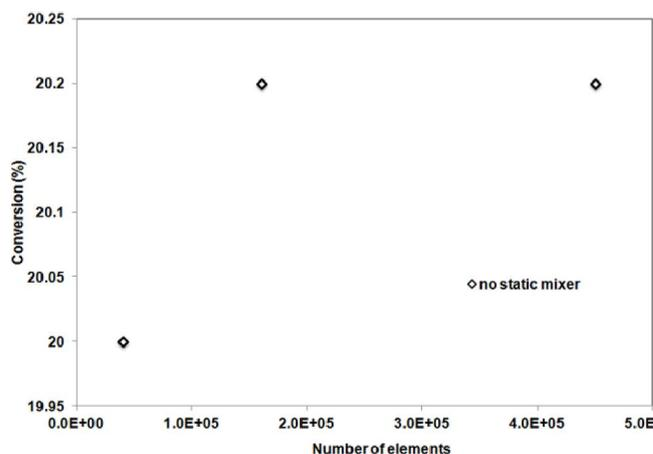
Figure 2 : Grid sensitivity test ( $Re = 0.1$ , channel without static mixer)
