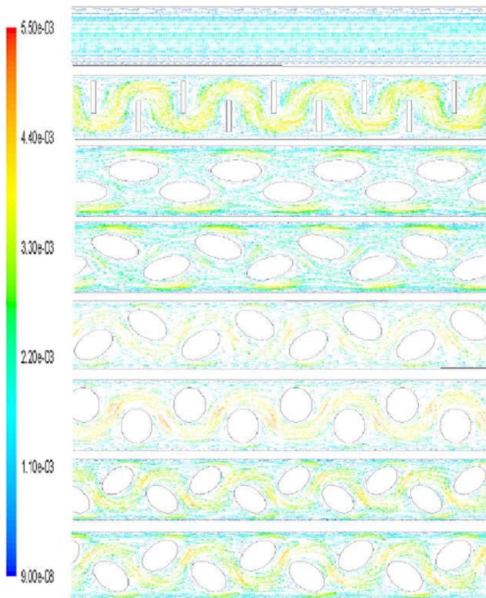
Figure 5 : Velocity vectors for  $Re = 0.1$
