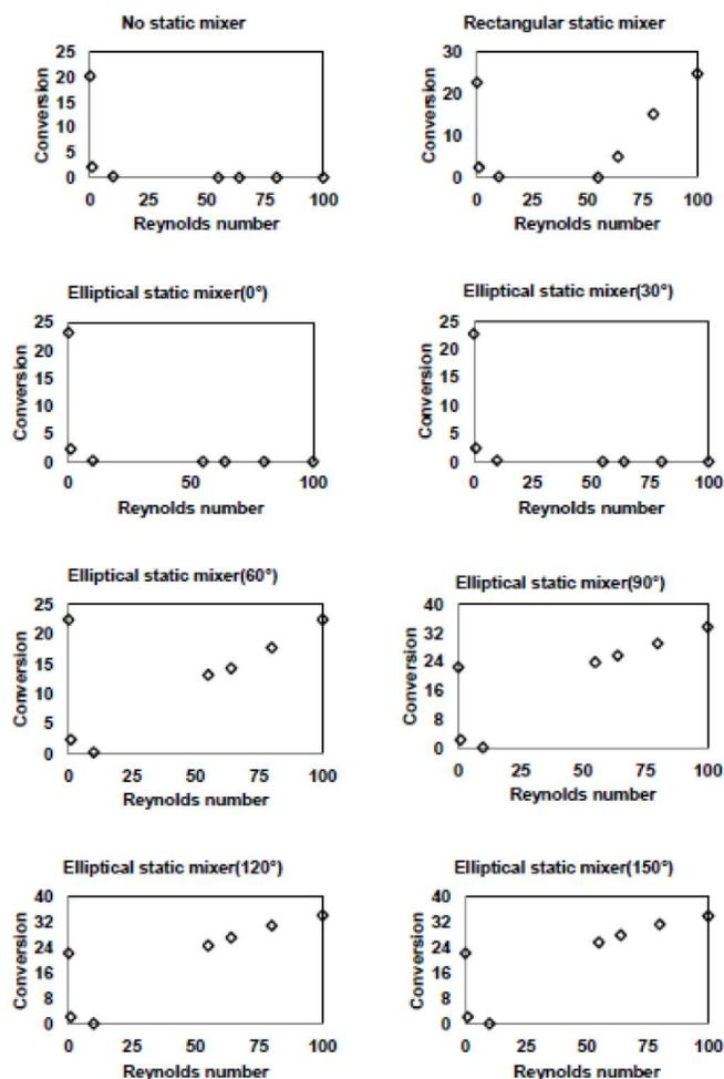
**Figure 6 : Effect of change in Reynolds number on conversion, in the presence and absence of mixers.**
