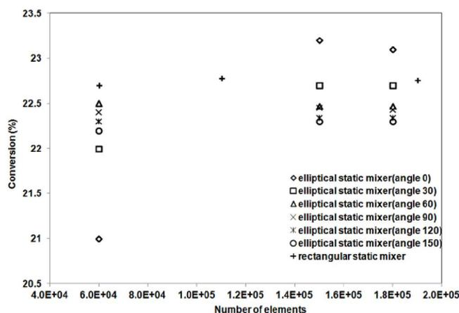
Figure 3 : Grid sensitivity test ( $Re = 0.1$ , channel with different static mixers)
