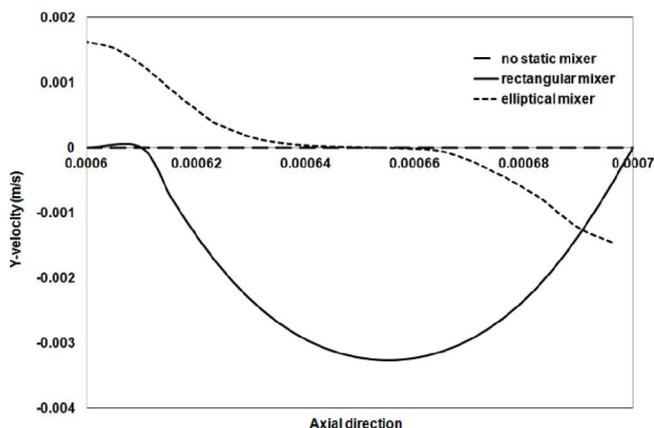
Figure 4 : Effect of mixers on lateral velocity. Simulation conditions  $Re = 0.1$ .
