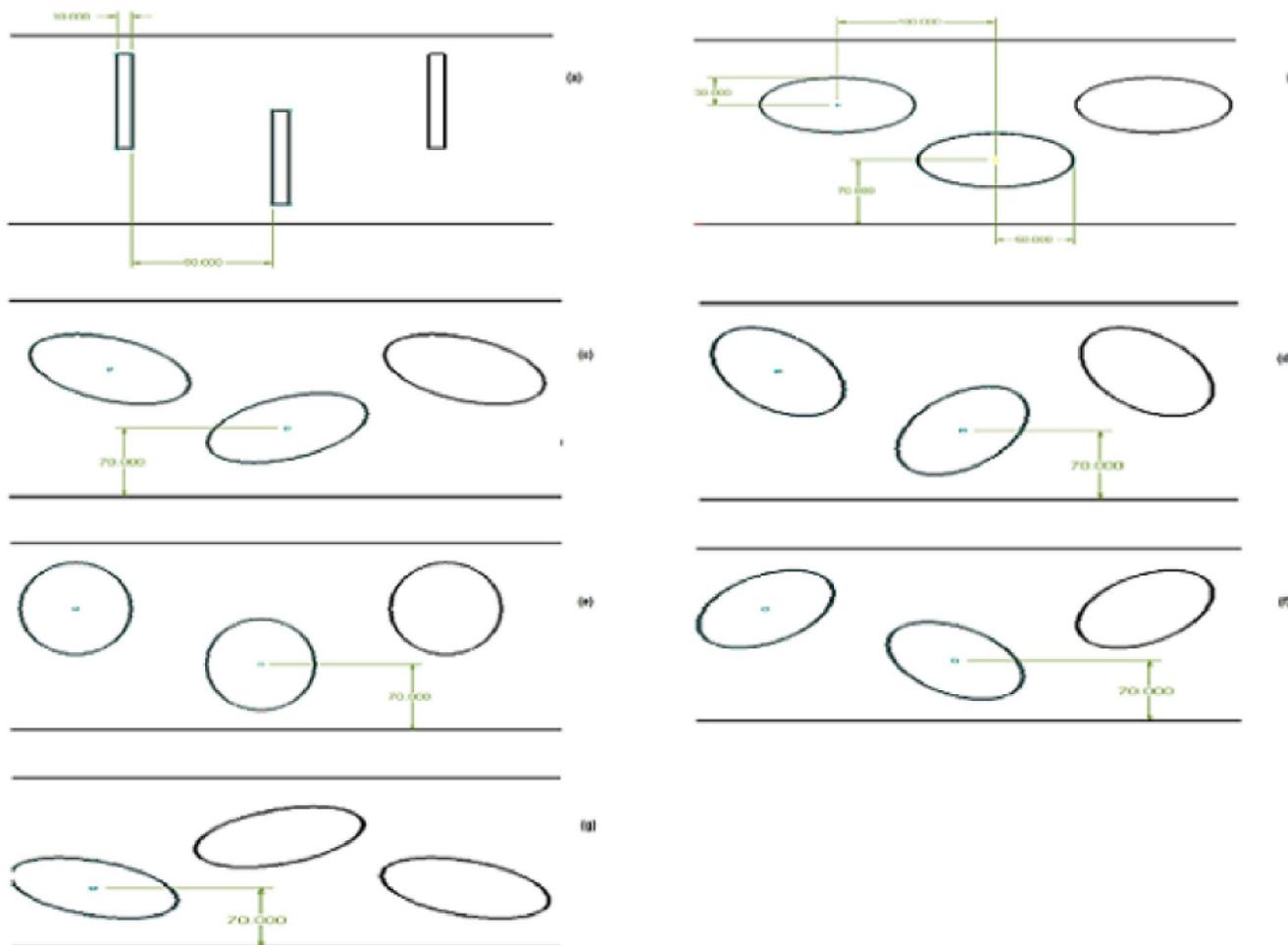
**Figure 1 :** Schematic of different static mixers shown over a section of the channel, a) rectangular static mixer, b) elliptical static mixer streamlined to the flow, c) elliptical static mixer at 30°, d) elliptical static mixer at 60°, e) elliptical static mixer at 90°, f) elliptical static mixer at 120°, g) elliptical static mixer at 150°.
