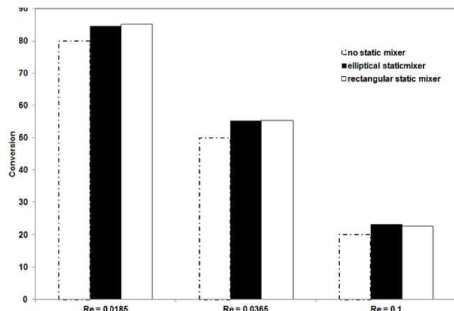
Figure 7 : Effect of mixers on conversion at lower Reynolds number.
