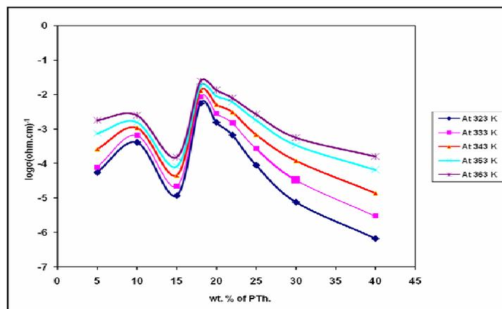
**Fig. 1: Variation of conductivity with different wt. % of thiophene at various temperatures**
