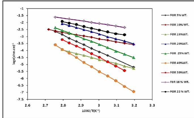
Fig. 3: Plot of variations of dc conductivity with temperature for different wt % of thiophene in PTh-PVAc films
