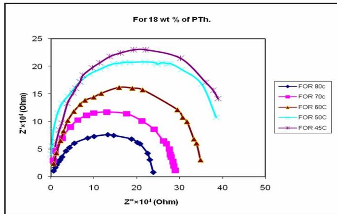
Fig.4: Nyquist plots  $Z'$  versus  $Z''$  at various temperature for 18 wt. % of thiophene
