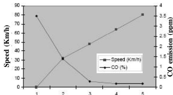
Figure 8: Correlation between speed and carbon monoxide emissions
