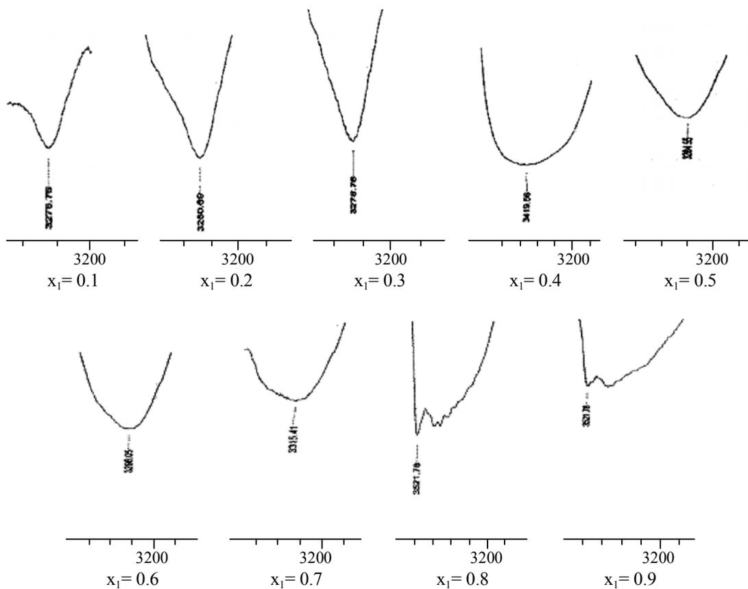
**Fig. 4:** IR stretching frequencies spectra of -OH (cm<sup>-1</sup>) for OCP + DN system
