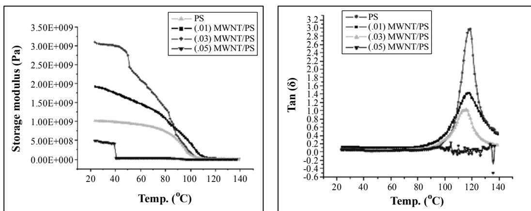
**Fig. 2: (a) Storage modulus vs temperature and (b) Loss factor vs temperature for MWNT/PS Nanocomposites**
