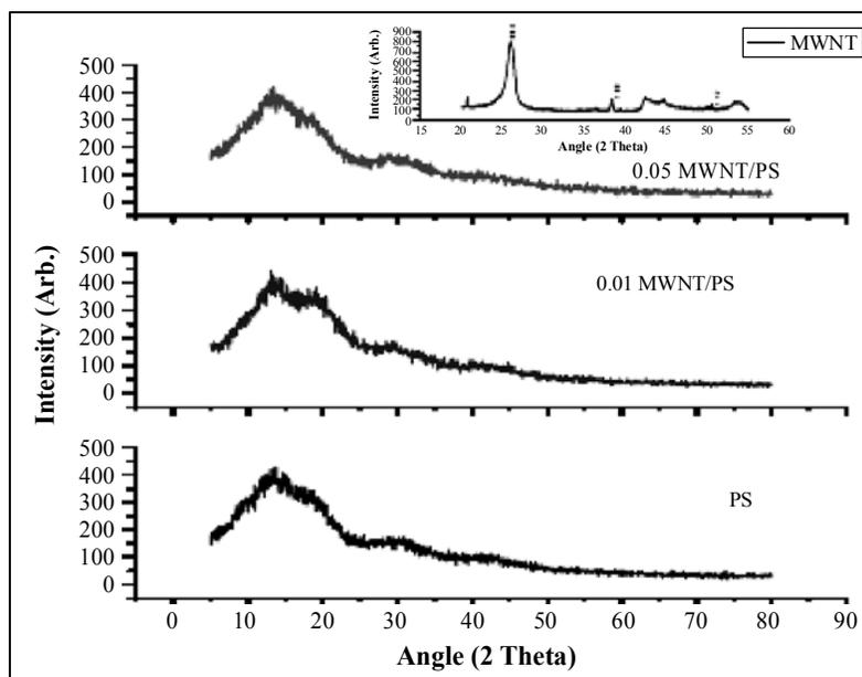
**Fig. 1: X-ray diffraction spectra for MWNT/PS nanocomposites**
