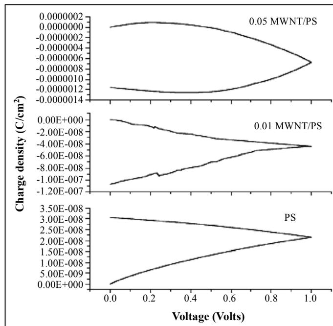
**Fig. 3: Cyclic Voltammetric response for MWNT/PS nanocomposites**
