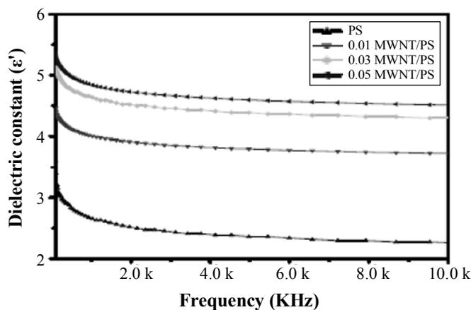
**Fig. 4: Frequency vs dielectric constant for MWNT/PS nanocomposites**
