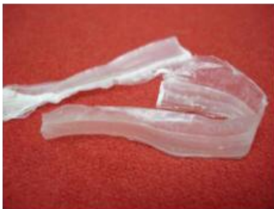
Figure 12 : Biodegradable plastic production after isolation, cloning and expression of Polyhydroxybutyrate genes in recombinant E. coli .
