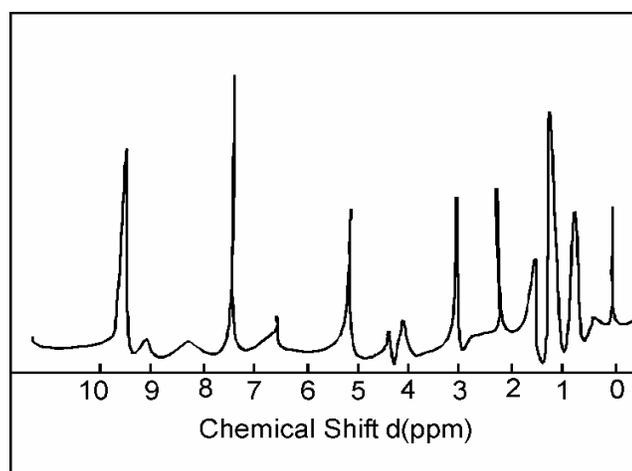
**Fig. 3: NMR Spectra of 8-HQ 5-ACF copolymer**
