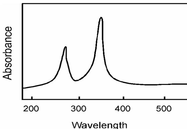
Fig. 1: UV-Visible spectra of 8-HQ 5-ACF copolymer
