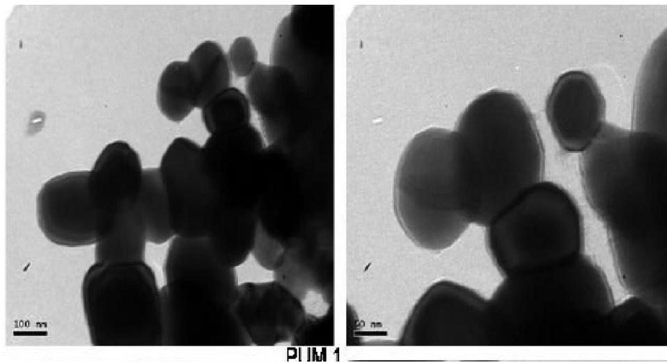
Figure 3 : TEM micrographs  $\text{Ni}_x\text{Zn}_{1-x}\text{Fe}_2\text{O}_4$  ferrites
