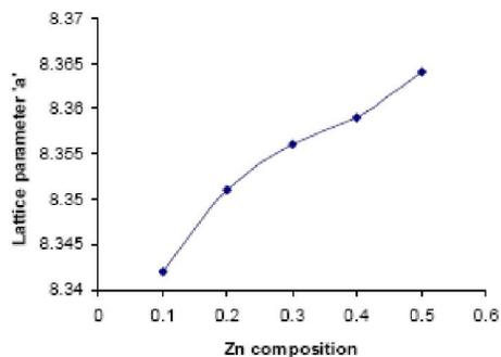
Figure 2 : Variation of lattice parameter with 'Zn' composition
