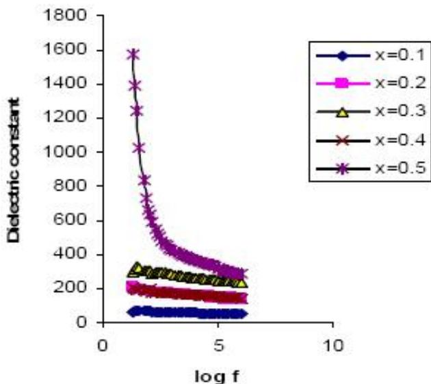
Figure 5 : Variation of dielectric constant with frequency
