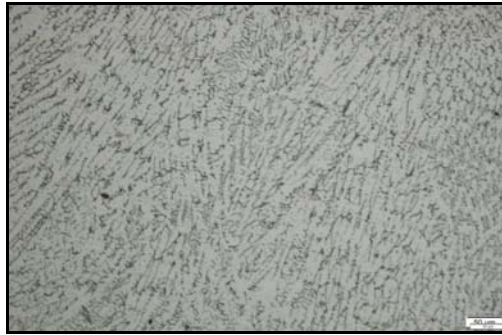
Fig. 5: Micro structure of weld area
