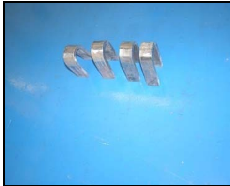
Fig. 2: Bend test specimens
