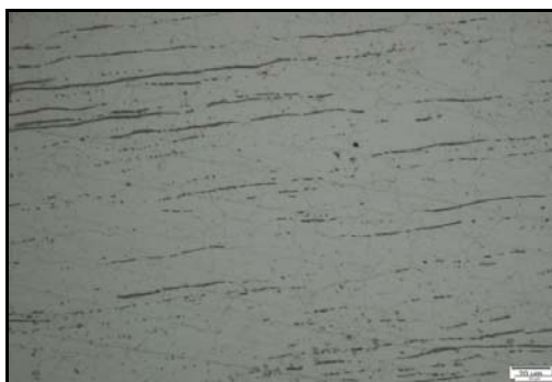
Fig. 4: Micro structure of base metal
