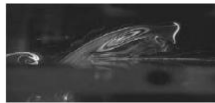
Figure 3: Smoke visualizations of vortex release from the cavity ( h_2/L=1 )
