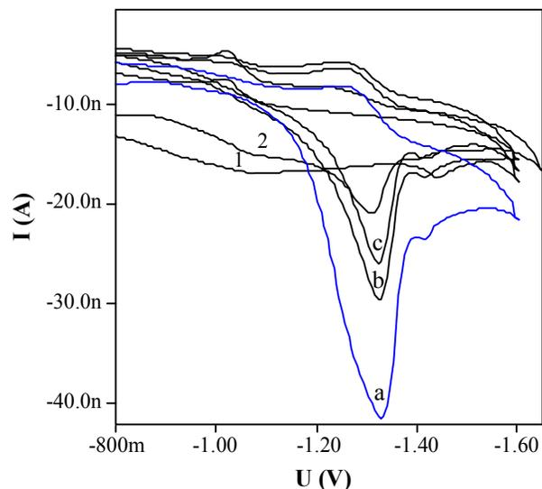
**Fig. 2: Cyclic voltammograms for  $10^{-7} \text{ mol.L}^{-1}$  atorvastatine (1) blank solution pH = 9.0; (2) without preconcentration  $t_{\text{acc.}} = 0 \text{ s}$ , (a) preconcentration for 60 s (b, c) repetitive cycle of (a, b respectively) at the same mercury drop; scan rate =  $100 \text{ mV s}^{-1}$  and  $E_{\text{acc.}} = -0.9 \text{ V}$**
