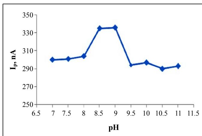
**Fig. 5: Effect of pH (7.0– 11.0) on the cathodic adsorptive stripping square-wave peak current of atorvastatine  $5 \times 10^{-7}$  mol. L<sup>-1</sup>,  $E_{acc.} = -0.5$  V,  $A=50$  mV,  $f = 50$  Hz**
