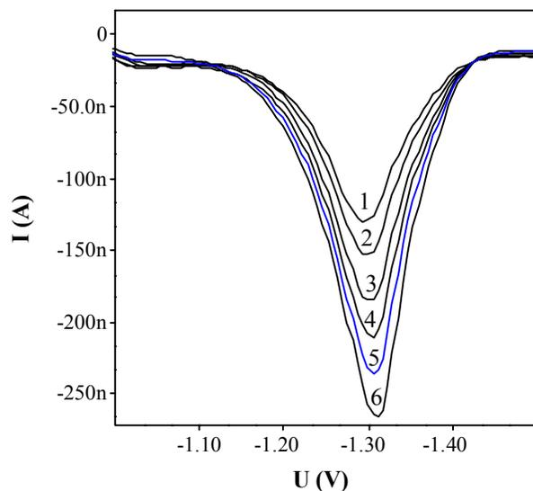
**Fig. 11: Cathodic adsorptive stripping square-wave voltammograms of atorvastatin in drug samples: (1)  $C_x$ , (2)  $C_x + 5 \times 10^{-8}$ , (3)  $C_x + 1.0 \times 10^{-7}$ , (4)  $C_x + 1.5 \times 10^{-7}$ , (5)  $C_x + 2.0 \times 10^{-7}$ , (6)  $C_x + 2.5 \times 10^{-7} \text{ molL}^{-1}$ ,  $E_{\text{acc.}} = -0.9 \text{ V}$ ,  $t_{\text{acc.}} = 30 \text{ s}$ ,  $a = 50 \text{ mV}$ ,  $f = 50 \text{ Hz}$  and BR buffer of  $\text{pH} = 9.0$**
