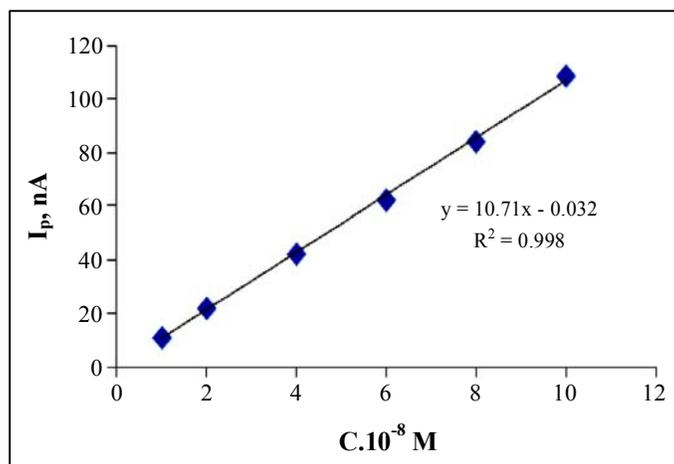
Fig. 8: Calibration of atorvastatin from  $1 \times 10^{-8}$  mol.L $^{-1}$  to  $1 \times 10^{-7}$  mol.L $^{-1}$
