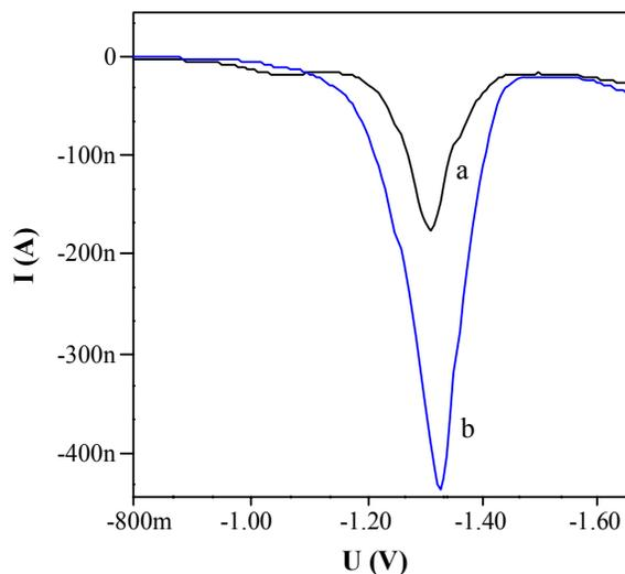
**Fig. 4: Square-wave (SW) adsorptive stripping voltammograms (SW) for  $2 \times 10^{-6} \text{ mol L}^{-1}$  atorvastatine in BR buffer of pH 9.0: (a)  $t_{\text{acc.}} = 0 \text{ s}$  and (b)  $t_{\text{acc.}} = 30 \text{ s}$ . Experimental conditions:  $E_{\text{acc.}} = -0.8 \text{ V}$ , pulse amplitude =  $50 \text{ mV}$ ,  $f = 100 \text{ Hz}$ , and  $\Delta E = 10 \text{ mV}$**
