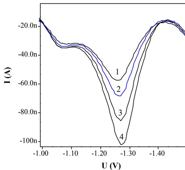
**Fig. 12: Cathodic adsorptive stripping square-wave voltammograms of atorvastatin spiked in plasma samples: (1) Atorvastatine  $1.0 \times 10^{-7}$ , (2)  $1.5 \times 10^{-7}$ , (3)  $2.0 \times 10^{-7}$ , (4)  $2.5 \times 10^{-7} \text{ molL}^{-1}$ ,  $E_{\text{acc.}} = -0.9 \text{ V}$ ,  $t_{\text{acc.}} = 30 \text{ s}$ ,  $a = 50 \text{ mV}$ ,  $f = 50 \text{ Hz}$  and BR buffer of  $\text{pH} = 9.0$**
