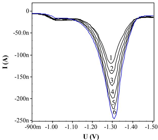
**Fig. 10: Cathodic adsorptive stripping square-wave voltammograms of atorvastatin in drug samples: (1)  $C_x$ , (2)  $C_x + 5 \times 10^{-8}$ , (3)  $C_x + 1.0 \times 10^{-7}$ , (4)  $C_x + 1.5 \times 10^{-7}$ , (5)  $C_x + 2.0 \times 10^{-7}$ , (6)  $C_x + 2.5 \times 10^{-7} \text{ mol.L}^{-1}$ ,  $E_{\text{acc.}} = -0.9 \text{ V}$ ,  $t_{\text{acc.}} = 30 \text{ s}$ ,  $a = 50 \text{ mV}$ ,  $f = 50 \text{ Hz}$  and BR buffer of  $\text{pH} = 9.0$**
