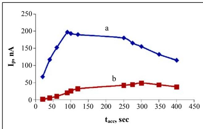
**Fig. 6: Effect of accumulation time ( $t_{acc}$ ) on the cathodic adsorptive stripping square-wave peak current of two different concentrations of atorvastatine: (a):  $5 \times 10^{-7} \text{ mol L}^{-1}$  and (b)  $10^{-8} \text{ mol L}^{-1}$ ,  $E_{acc} = -0.4 \text{ V}$ ,  $a = 50 \text{ mV}$ ,  $f = 50 \text{ Hz}$**
