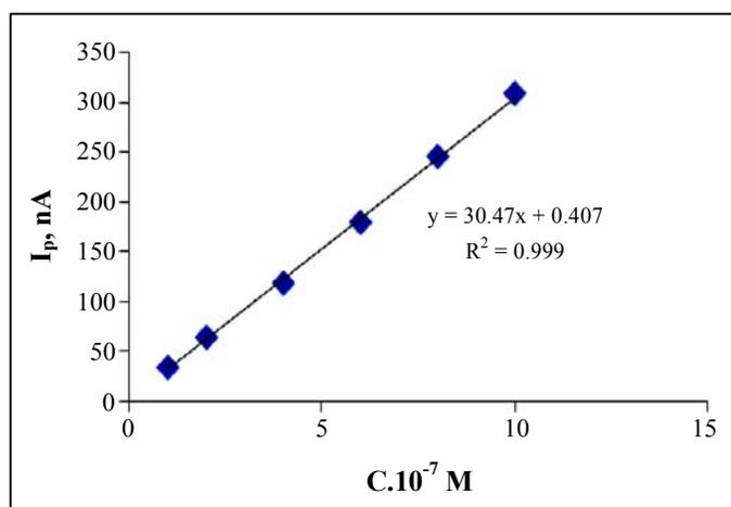
Fig. 9: Calibration of atorvastatin from  $1 \times 10^{-7}$  mol.L $^{-1}$  to  $1 \times 10^{-6}$  mol.L $^{-1}$
