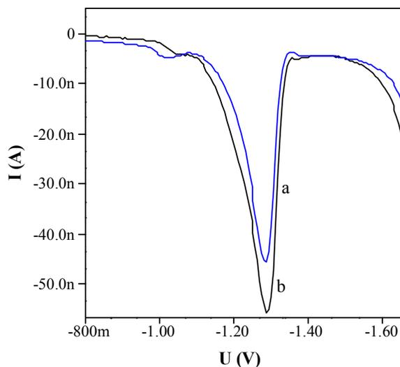
**Fig. 3:** Differential pulse (DP) adsorptive stripping voltammograms for  $2 \times 10^{-6} \text{ mol L}^{-1}$  atorvastatine in BR buffer of pH 9.0: (a)  $t_{\text{acc.}} = 0 \text{ s}$  and (b)  $t_{\text{acc.}} = 30 \text{ s}$ . Experimental conditions:  $E_{\text{acc.}} = -0.8 \text{ V}$ , pulse height =  $50 \text{ mV}$ , and scan rate =  $10 \text{ mV s}^{-1}$
