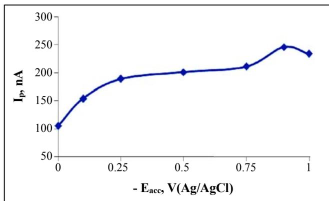
**Fig. 7: Effect of accumulation potential ( $E_{acc}$ ) on the cathodic adsorptive stripping square-wave peak of atorvastatine  $5 \times 10^{-7} \text{ mol L}^{-1}$ ,  $a = 50 \text{ mV}$ ,  $f = 50 \text{ Hz}$**
