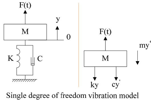
Figure 1: A single degree of freedom vibration model
