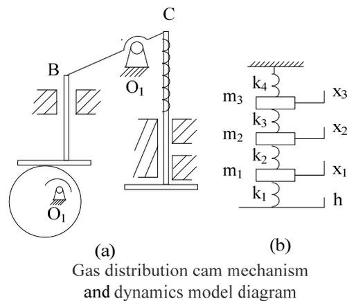
Figure 8 : An engine cam mechanism system
