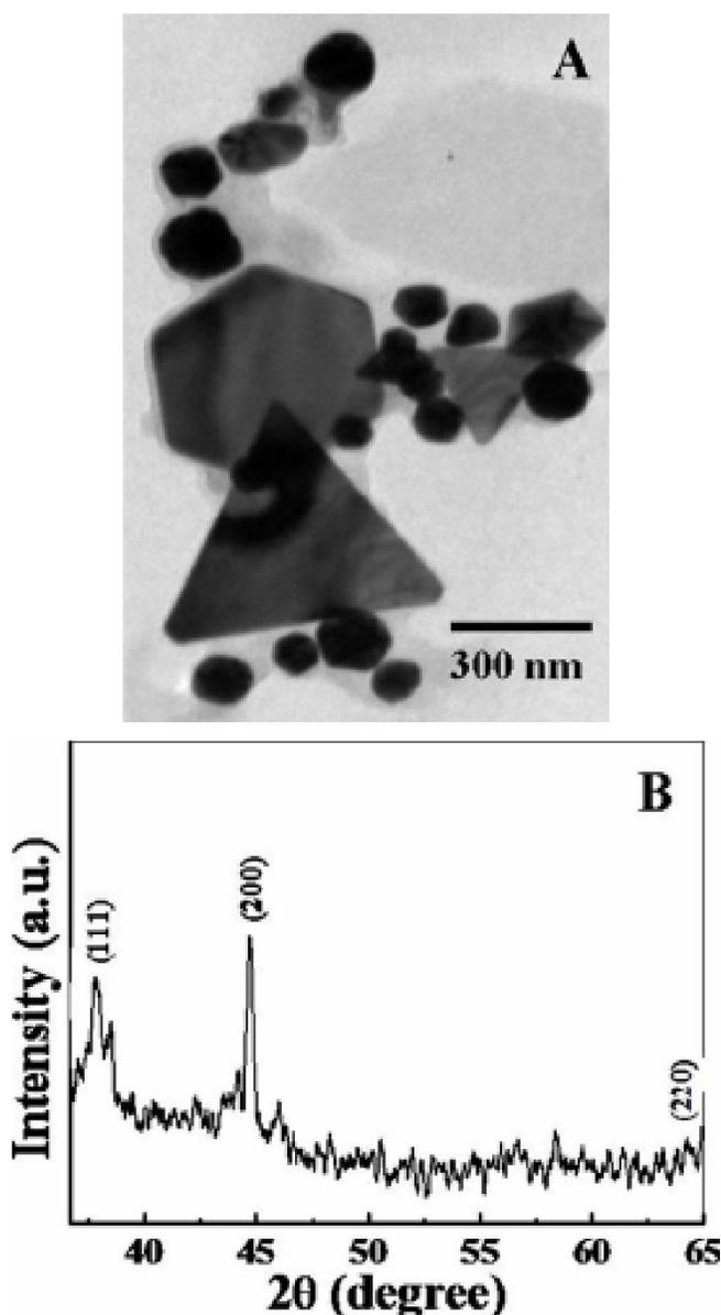
Figure 2 : Representative TEM image of TC leaf extract-reduced silver nanoparticles (A). (B) XRD pattern of a solution-cast film of the TC leaf extract-reduced silver nanotriangles deposited on a glass substrate. The Bragg reflections are identified in the XRD pattern.
