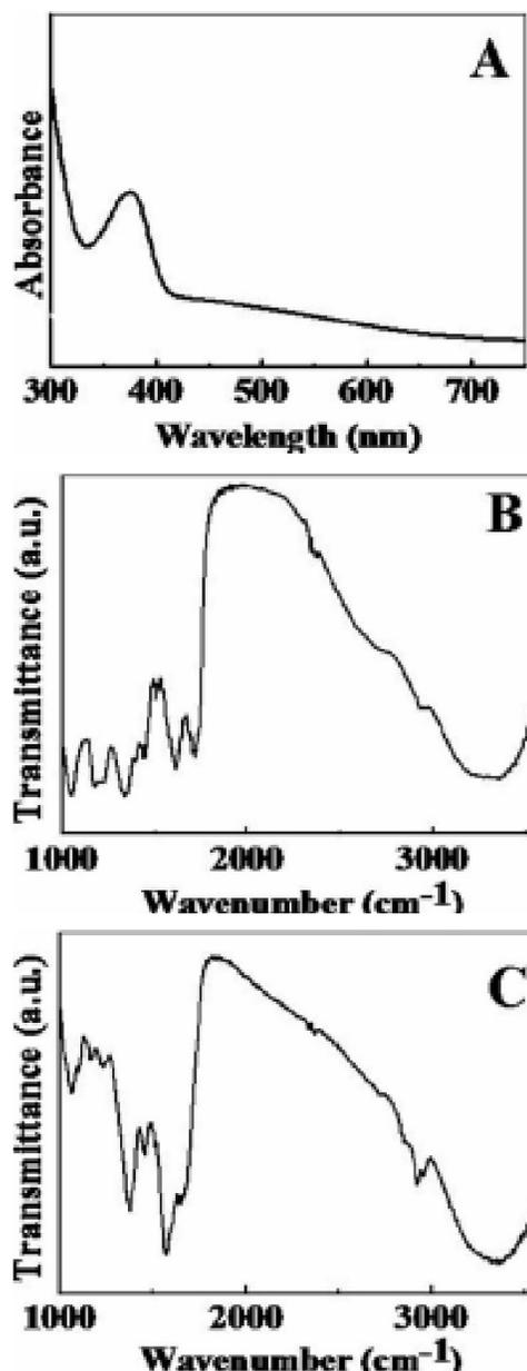
Figure 1 : A UV-vis absorption spectra recorded TC leaf extract-reduced silver nanoparticles; FTIR spectra recorded (B) from pure TC leaf extract and (C) from TC leaf extract-reduced silver nanoparticles.
