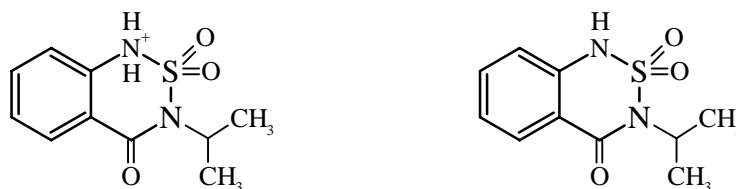
Fig. 4: Structural formula of bentazon at low pH (left), and at high pH (right), as theoretically expected to be positively charged at low pH due to the presence of secondary and tertiary amine.
