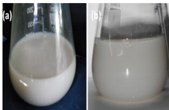
FIG.3. Biosynthesis of silver nanoparticle using Bacillus sp. (a) with addition of cadmium sulphate 12 h incubation (b) 24 h incubation.
